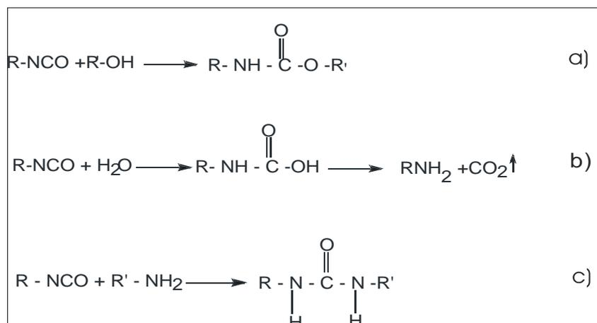
**Figure 1.** Isocyanate reactions with alcohol (a) and with water (b,c).
