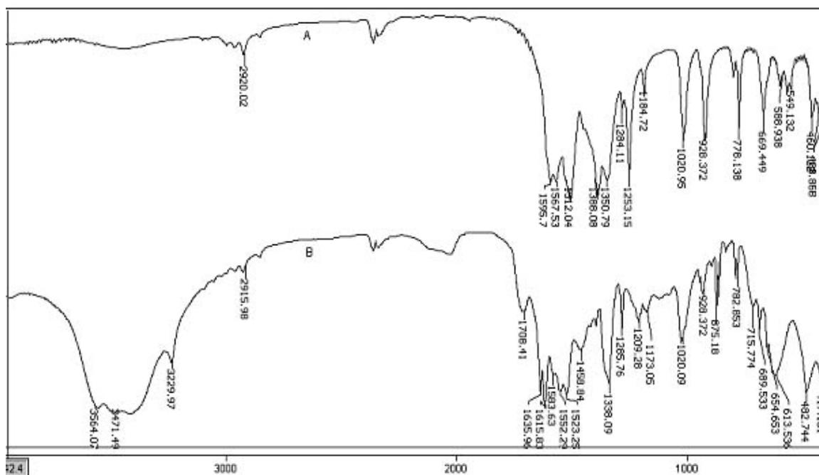
**Figure 1.** Comparative FTIR spectra: A) the complex of Mn(III)-acetylacetonate, B) the complex of Mn(III)-diacetylacetonemaleate.
