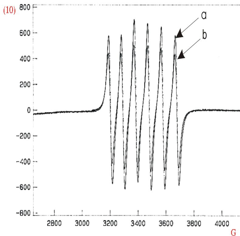
**Figure 7.** The comparison of the ESR spectra after the balance has been established of  $\text{Mn}^{3+}/\text{Mn}^{2+}$  a) of Mn(III)-diacetylacetonemaleate, and b) of Mn(III)-diacetylacetonehydroxylaminmaleate.
