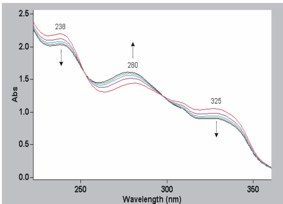
**Figure 6.** The UV spectra of the decomposition of the complex of Mn(III)-diacetylacetonehydroxylaminmaleate in ethanol with respect to time (15 min).
