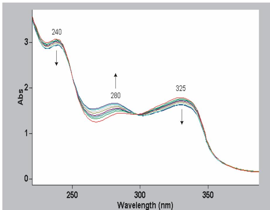
**Figure 4.** The UV spectra of the decomposition of the complex of Mn(III)-diacetylacetonemaleate in ethanol with time (30 min.).
