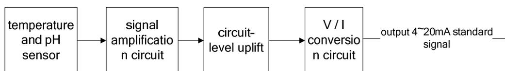
In the designing the transmitter, how much the signal shall be amplified and how high the electrical level shall be raised can all be adjusted according to the practical needs. The output signal of several types of sensors can be switched to the 0–3 V range and 4–20 mA standard electric current output as signals. This flexible design enables the monitoring nodes to adapt to all kinds of sensors with different settings.
