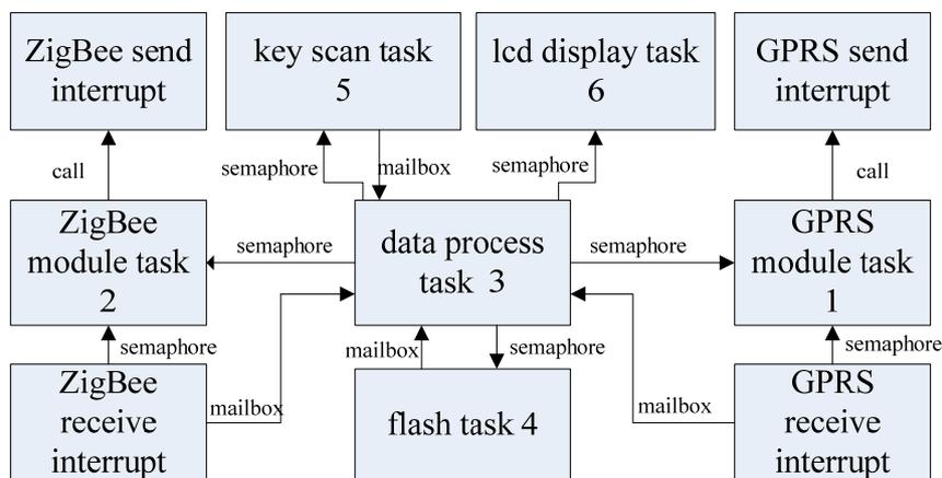
The other tasks and interrupt service subroutine deliver the message and the keys to the data process task, and the data process task notifies the other tasks to deal with the message. The other tasks and interrupt service subroutine communicate with the data process task through a unified message
