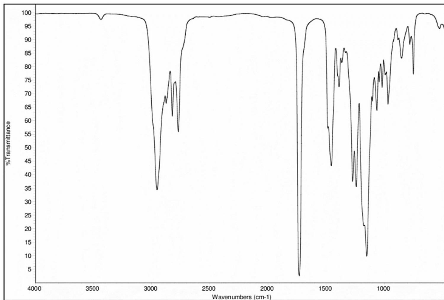
Figure S3. IR SPECTRUM OF COMMERCIAL EUDRAGUARD CONTROL (EUG-C) (source: Evonik website)
