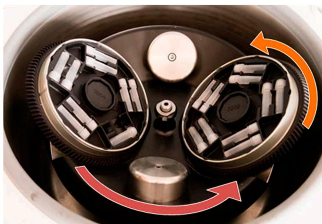
**Figure 1.** Design of the dual centrifuge ZentriMix with adapters for 2 mL tubes. The rotation around the central axis is indicated in red. Marked in orange is the second axis around which the sample tubes are rotated. Modified from [21].
