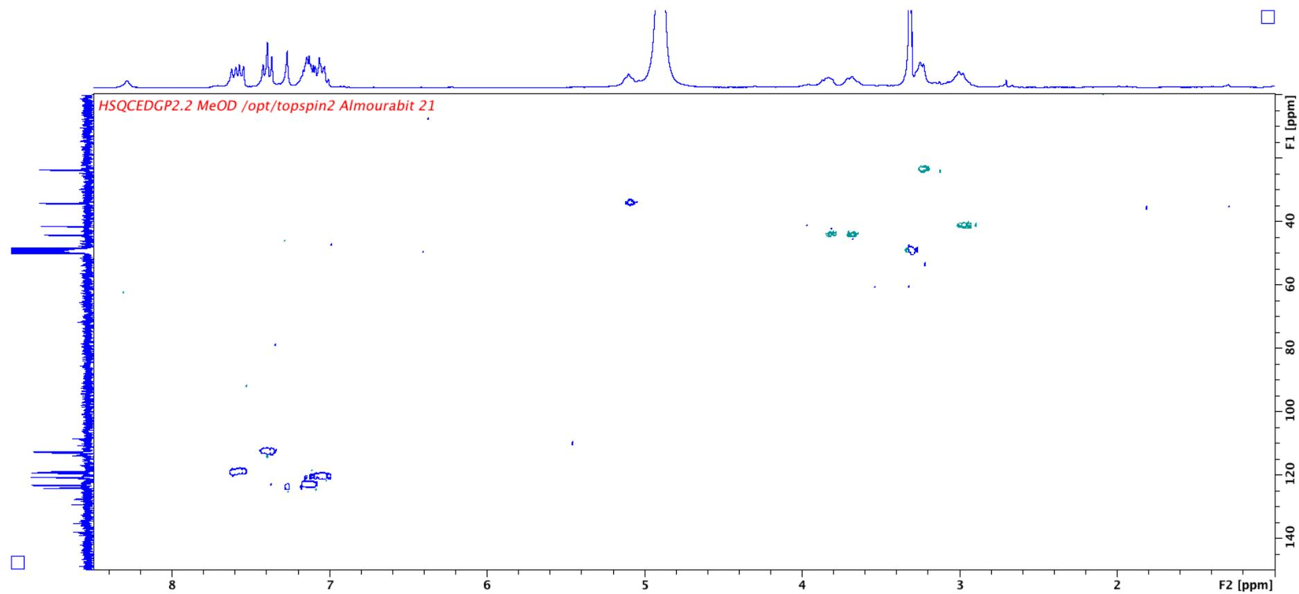
Figure S6:  $^1\text{H}$ - $^{13}\text{C}$  HMBC NMR (300 MHz, MeOD) spectrum for 6,6'-bis-(debro)-gelliusine F (1)
