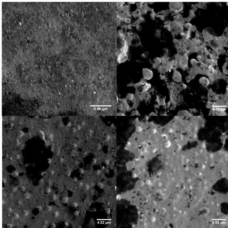
**Figure 6.** Scanning electron microscope images of nanocomposites prepared with LMW CS solutions at 10<sup>-5</sup> g/mL (upper left) or at 10<sup>-7</sup> g/mL (upper right), or MMW CS solutions at 10<sup>-5</sup> g/mL (lower left) or at 10<sup>-7</sup> g/mL (lower right). All images were made at a magnification of 2000×. The scale bars in the images represent 4.52 µm.
