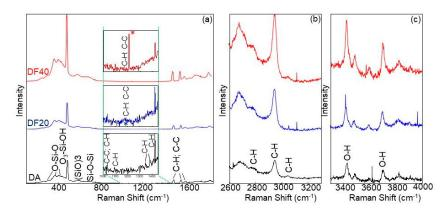
**Figure 2.** Raman spectra of DA (black line), DF20 (blue line) and DF40 (red line) in three different ranges: (a) 80–2000 cm<sup>-1</sup>, (b) 2600–3300 cm<sup>-1</sup>, and (c) 3300–4000 cm<sup>-1</sup>. Insets in (a) show the corresponding 1000–1450 cm<sup>-1</sup> zoomed area, with blue and red asterisks indicating additional bands due to C-H and C-C bonds that appear after functionalization. Bonds involved in Raman bands are also reported.
