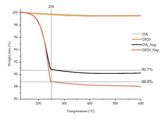
Figure 6. Thermograms for DA, DA\_Nap, DF20 and DF20\_Nap.
