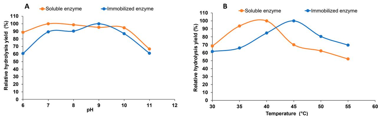
**Figure 3.** Effect of varying reaction conditions: (A) pH range from pH 6–11 and (B) temperature (30–55 °C) in the hydrolysis of sodium alginate by soluble and immobilized enzyme.
