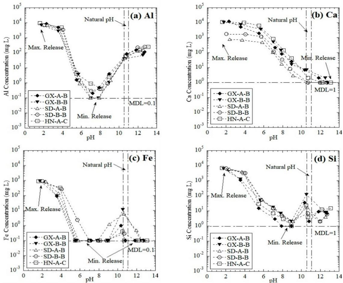
**Figure 3.** Leaching of major elements as a function of pH from red mud: (a) Al, (b) Ca, (c) Fe, and (d) Si. MDL = method detection limit.
