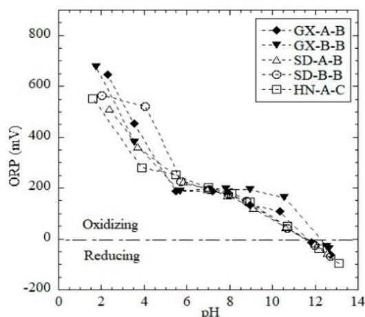
**Figure 2.** Oxidation-reduction potential as a function of pH in the eluate of pH-dependent leaching tests.
