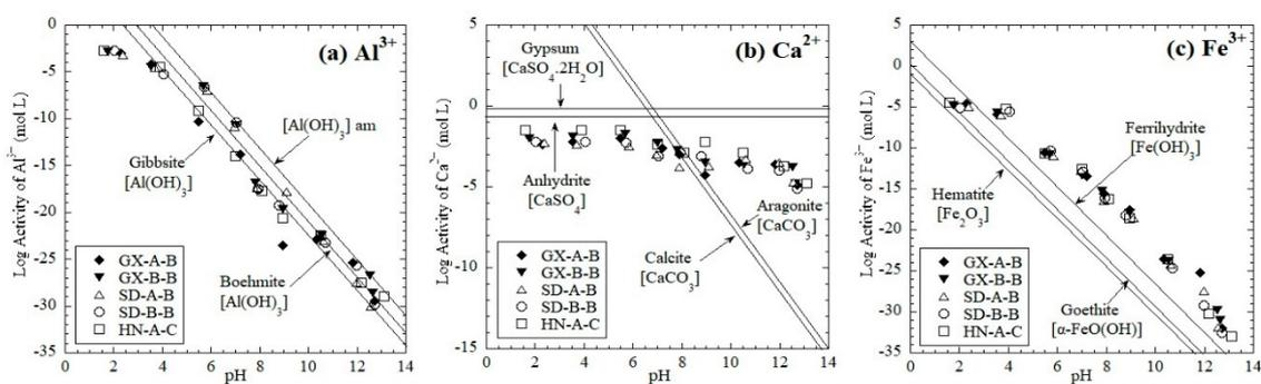
**Figure 6.** Log activity of major elements as a function of pH graphs: (a)  $\text{Al}^{3+}$ , (b)  $\text{Ca}^{2+}$ , and (c)  $\text{Fe}^{3+}$ .
