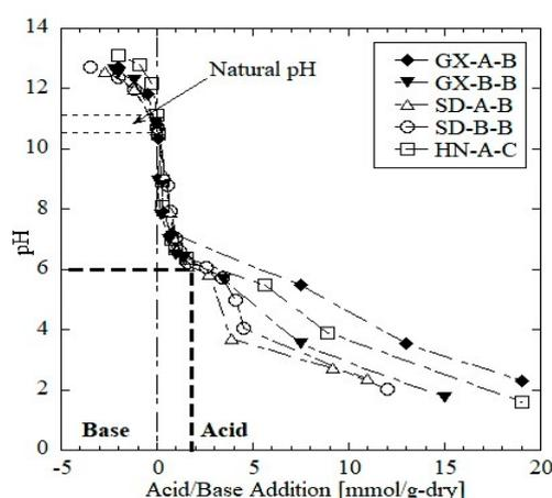
**Figure 1.** Acid neutralization capacity curves of red mud samples.
