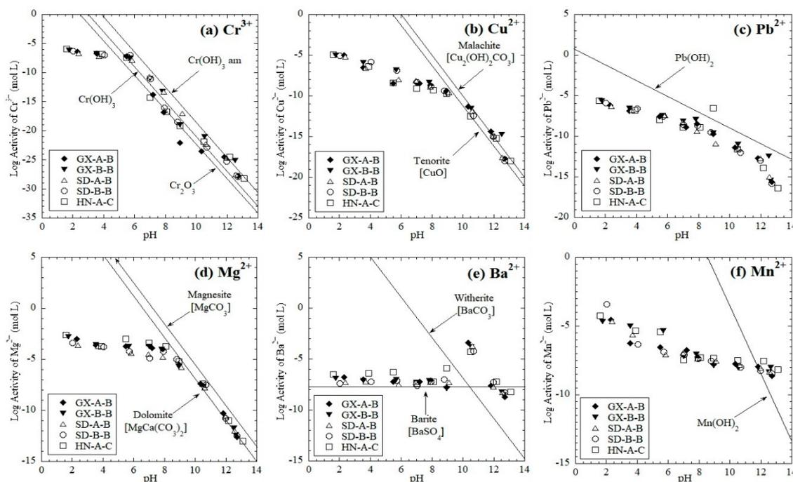
**Figure 7.** Log activity of trace metals as a function of pH (a)  $\text{Cr}^{3+}$ , (b)  $\text{Cu}^{2+}$ , (c)  $\text{Pb}^{2+}$ , (d)  $\text{Mg}^{2+}$ , (e)  $\text{Ba}^{2+}$ , and (f)  $\text{Mn}^{2+}$ .
