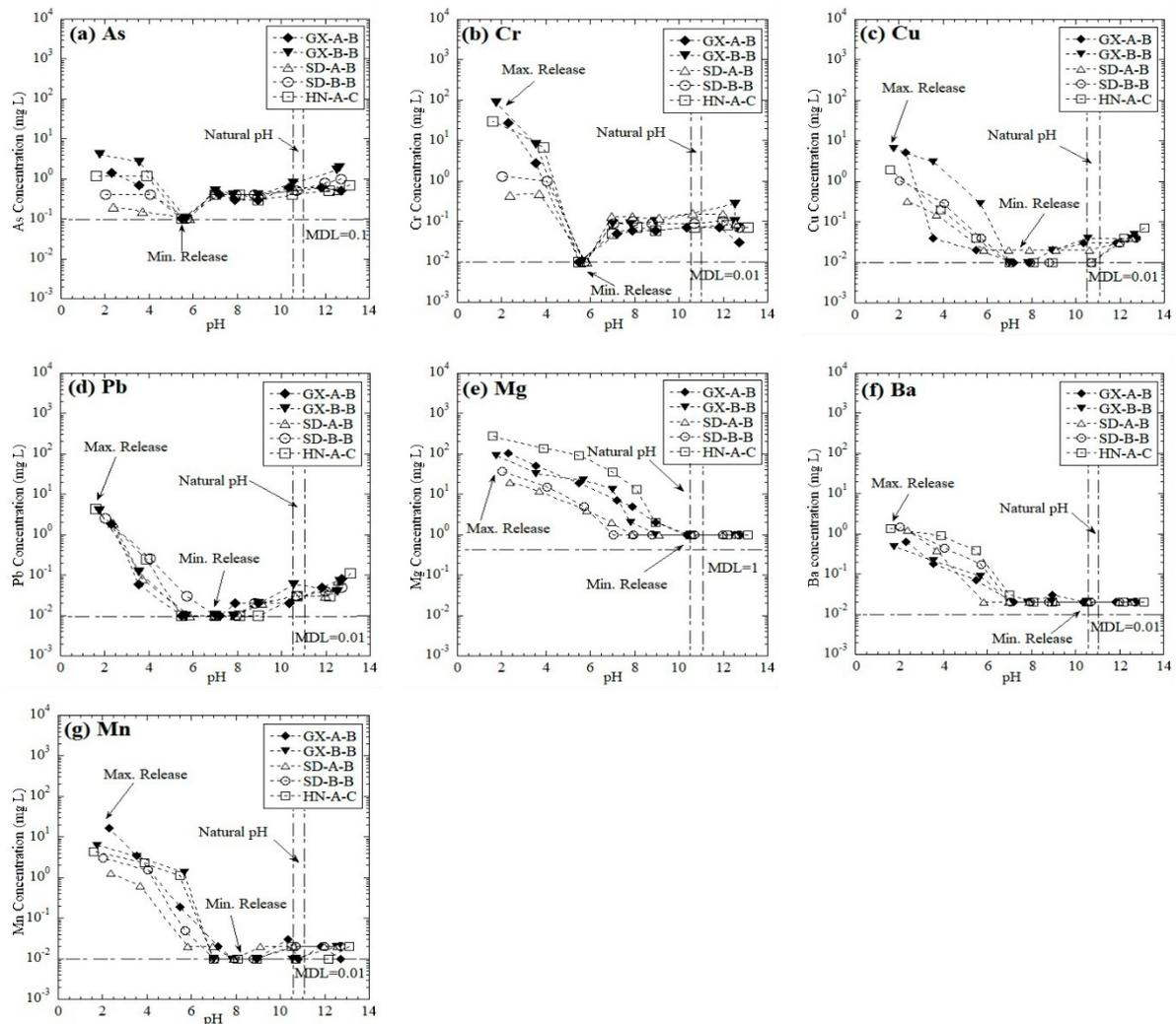
**Figure 4.** Leaching of trace elements as a function of pH from red mud: (a) As, (b) Cr, (c) Cu, (d) Pb, (e) Mg, (f) Ba, and (g) Mn. (MDL means method detection limit).
