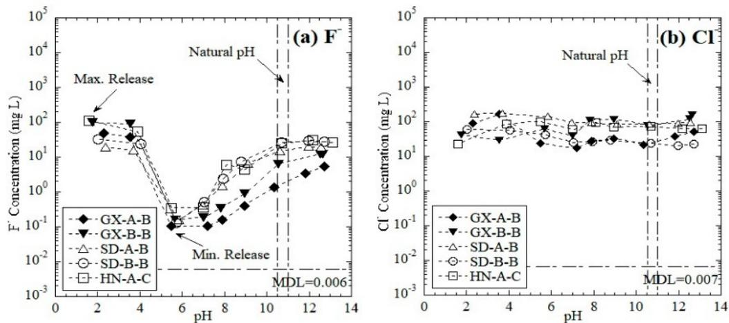
**Figure 5.** Leaching of toxic anions as a function of pH from RM: (a)  $F^-$  and (b)  $Cl^-$ . MDL = method detection limit.
