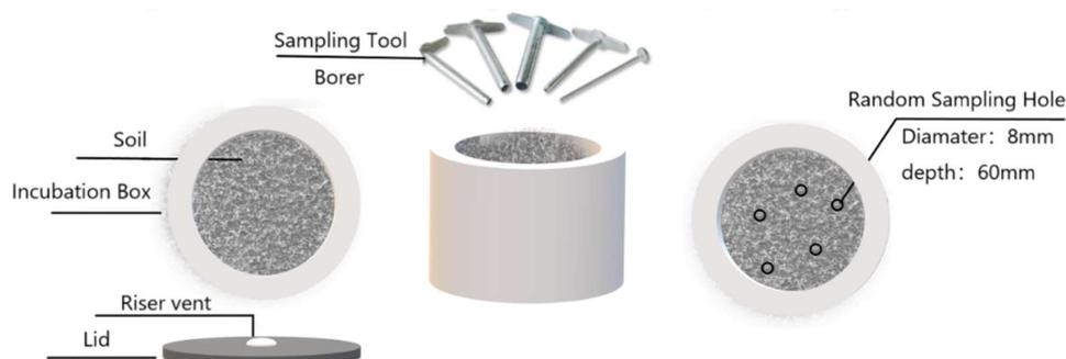
**Figure 1.** Abridged general view of soil sampling. Five random vertical sampling holes (diameter: 8 mm; depth: 60 mm) were implemented for lessening the disturbance of sampling to microbes.
