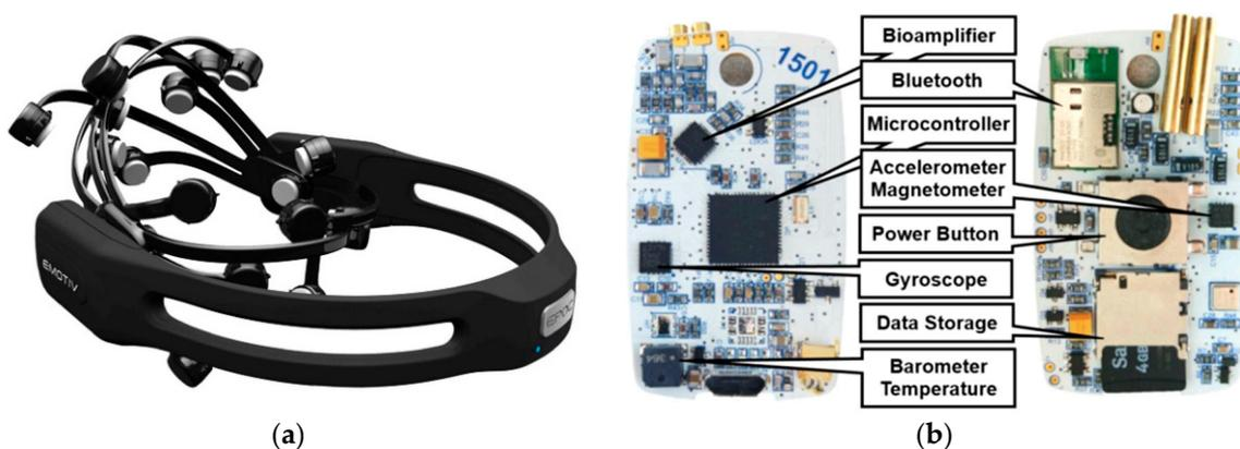
**Figure 3.** Emotiv Eloc helmet (a) and designed ECG holler (b).
