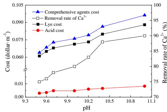
Figure 4. Dosage and cost of the chemicals used in the system under different pH conditions.
