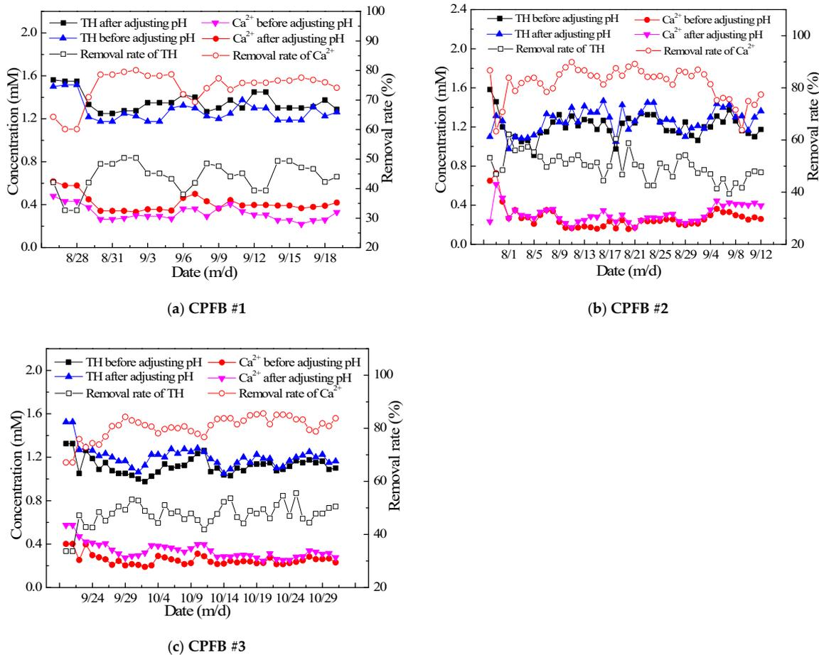
**Figure 3.** Hardness and  $\text{Ca}^{2+}$  ion removal performance of circulating pellet fluidized beds (CPFBS). ((a)-hardness and  $\text{Ca}^{2+}$  ion removal performance of circulating pellet fluidized bed(CPFBS) #1 at different dates; (b)-hardness and  $\text{Ca}^{2+}$  ion removal performance of circulating pellet fluidized bed(CPFBS) #2 at different dates; (c)-hardness and  $\text{Ca}^{2+}$  ion removal performance of circulating pellet fluidized bed(CPFBS) #3 at different dates).
