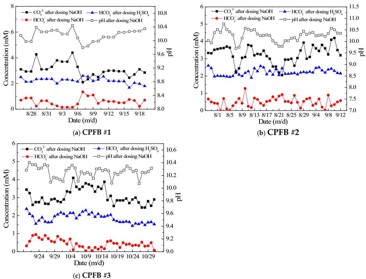
Figure 5. Alkalinity removal performance of the CPFBs. ((a)-alkalinity removal performance of the circulating pellet fluidized bed(CPFB) 1# at different dates; (b)-alkalinity removal performance of the circulating pellet fluidized bed(CPFB) 2# at different dates; (c)-alkalinity removal performance of the circulating pellet fluidized bed(CPFB) 3# at different dates).
