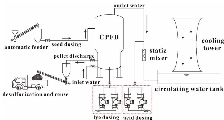
**Figure 1.** Flow chart of the circulating pellet fluidized bed softening system.
