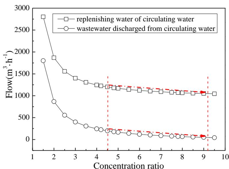
**Figure 7.** Amount of water replenished to and amount of wastewater discharged from the circulating water system for different concentration ratios.
