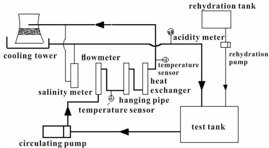
Figure 2. Flow chart of the dynamic scale-inhibition simulation test.
