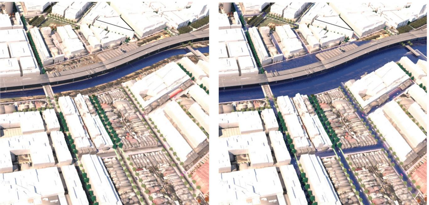
**Figure 16.** Detail rendering, aerial view looking east for scenario (2) road-based integrated water management LEFT under dry conditions and RIGHT under flood conditions. Image by authors using multi-criteria street tree design decision support modelling approach in Autodesk™ 3ds Max™.
