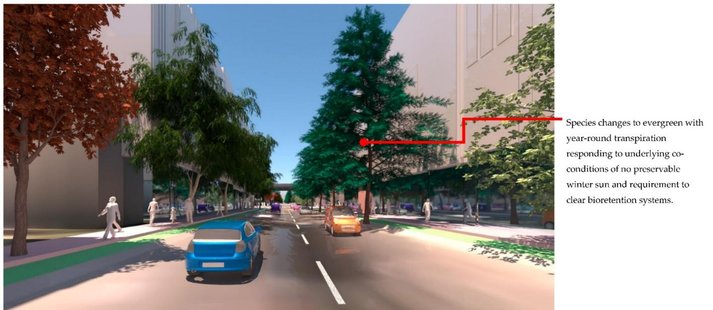
**Figure 18.** Macaulay Road view of Flood scenario (2) ‘road-based integrated water management’ during dry weather. In both schemes trees on the right-hand side are positioned in the road just beyond the bike path to achieve the summer active transport objective. Image by authors using multi-criteria street tree design decision support modelling approach in Autodesk™ 3ds Max™.
