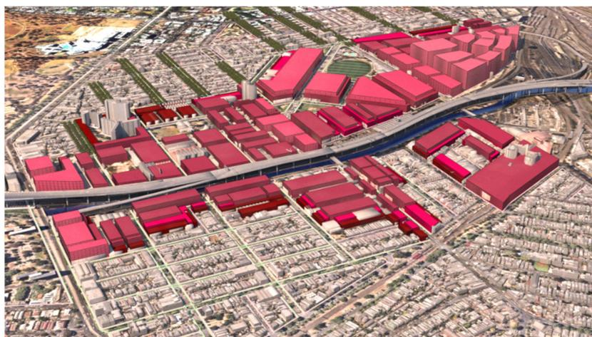
**Figure 4.** Massing model of maximum building envelopes regulated in the C190 amendment: dark red, 10.5 m interfacing residential areas; pale pink, height restrictions up to 60 m. Image by authors using multi-criteria street design decision support modelling approach in Autodesk™ 3ds Max™.
