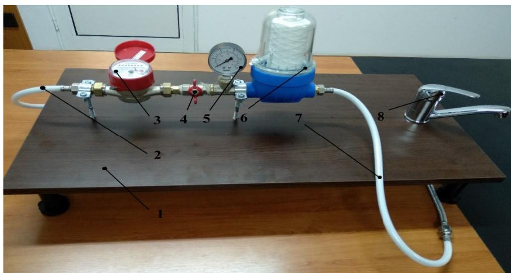
**Figure 2.** Experimental stand for testing the drinking water filters.
