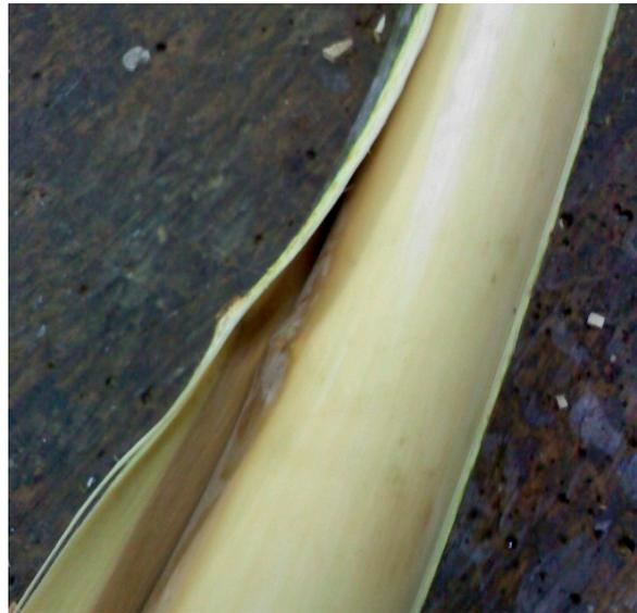
**Figure 1.** Mechanical bark separation.
