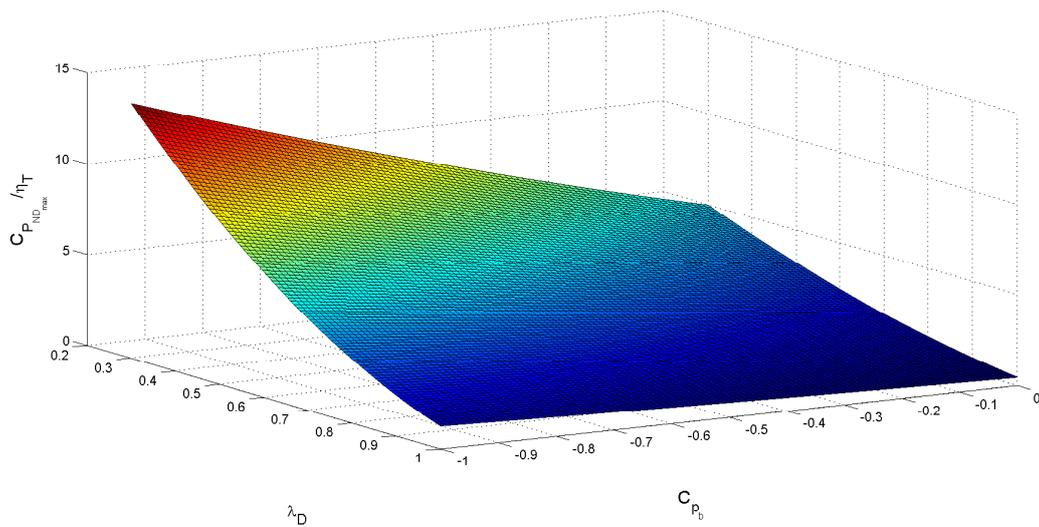
Figure 16. The maximum power coefficient as a function of back pressure and diffuser area ratio.
