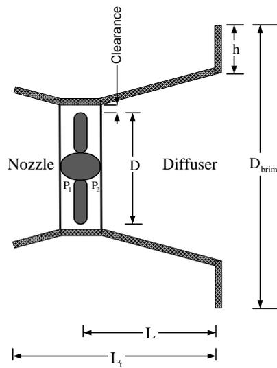
Figure 2. Wind turbine equipped with a brimmed diffuser [6].
