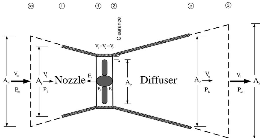
Figure 1. Stream tube passing through a shrouded wind turbine with nozzle and diffuser.
