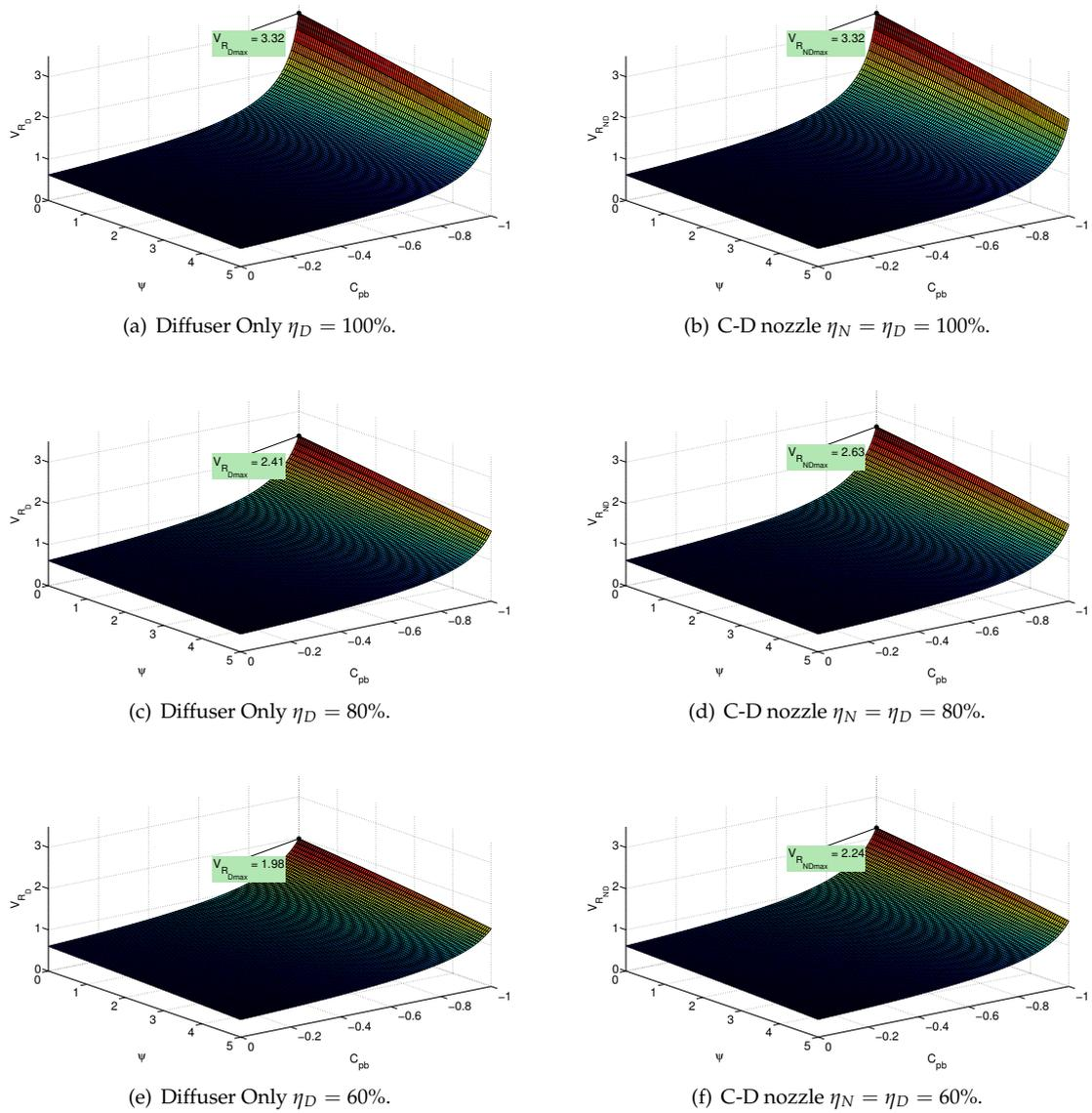
**Figure 7.** The effect of the pressure and loading coefficients on the velocity distribution of diffuser only and and converging-diverging (C-D) nozzle.
