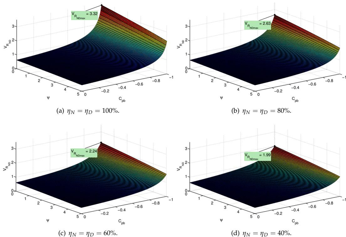
**Figure 10.** Plot of relative velocity ratios using  $D_i = 0.76$  m,  $D_1 = 0.7$  m and  $D_e = 1.072$  m for different efficiencies using Equation (33).
