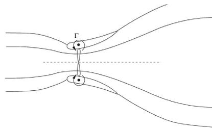
**Figure 5.** The duct shape used in Hansen's study [18].
