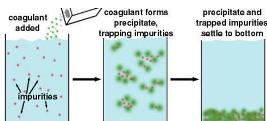
Figure 2. Coagulation/flocculation process [5].
