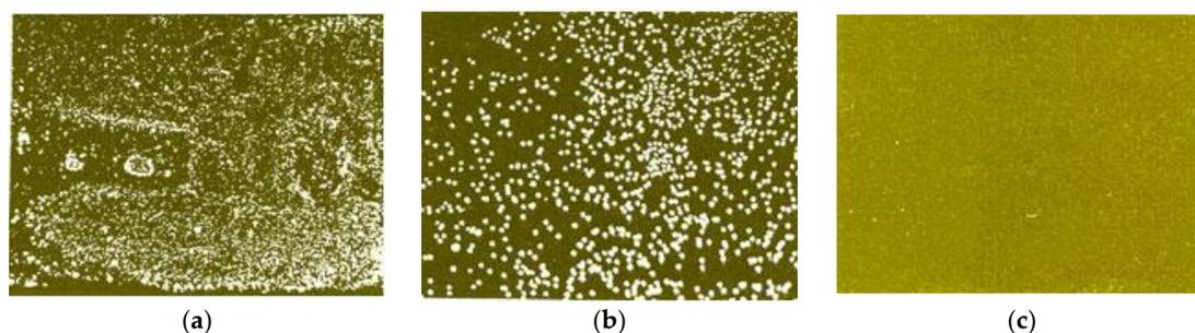
**Figure 1.** (a) Uncleaned (rinsed only), many bacterial colonies; (b) after chemical cleaning, reduced numbers of bacterial colonies; and (c) after cleaning and disinfection, very few bacterial colonies remain [4].
