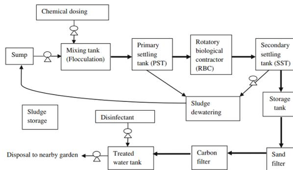
Figure 3. Process flow diagram of a small WWTP [94].
