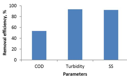
Figure 6. Removal efficiency of the combination of ferric chloride and chitosan.
