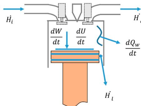
Figure 4. The thermodynamic process of the combustion chamber.
