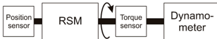
Figure 2. Block model of coupling for purposes of torque measurement.
