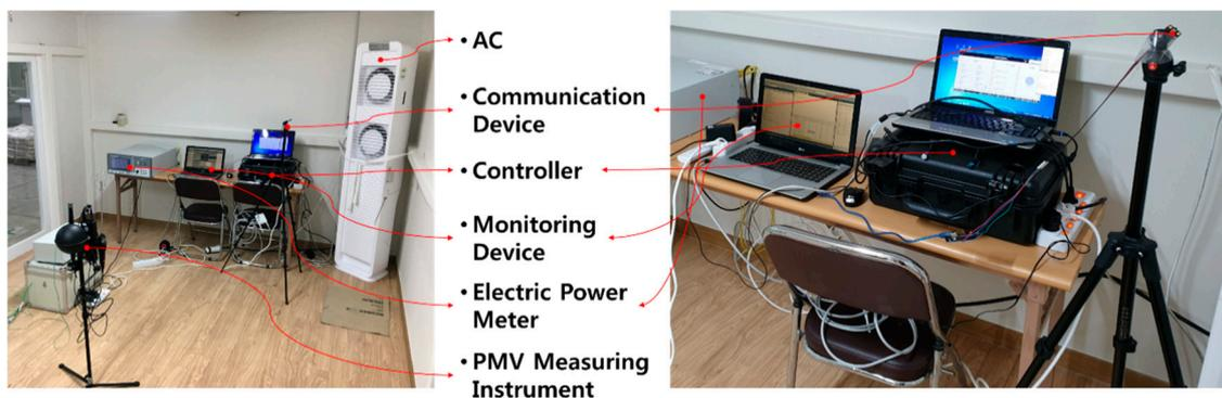
**Figure 13.** Air conditioner (AC) unit, TCC-V1, PMV meter installation status in the inner chamber.
