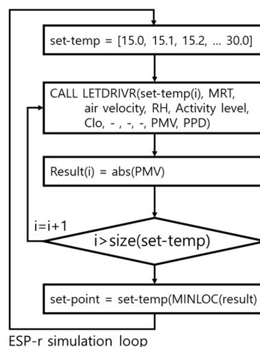
Figure 3. Analysis sequence in ESP-r for the calculation of the optimal temperature.
