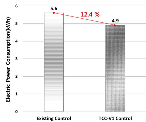
Figure 22. Comparison of electric energy consumption without and with TCC-V1 on October 17.
