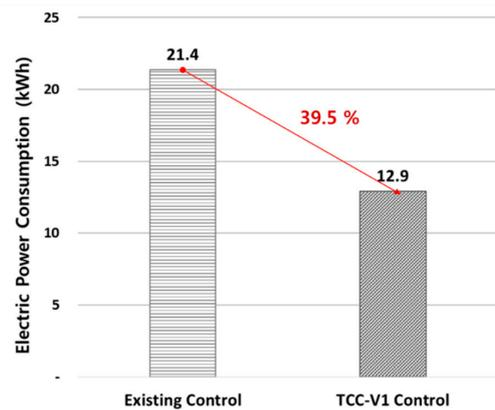
Figure 20. Comparison of electric energy consumption with and without TCC-V1 control on August 10.
