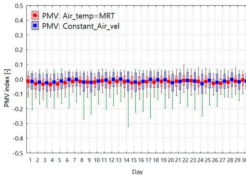
Figure 12. Daily PMV error in two scenarios with optimal setpoint of base case.
