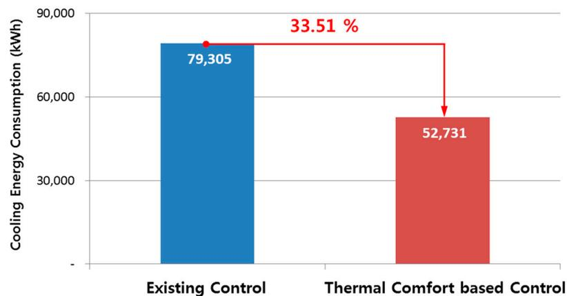
Figure 6. Cooling energy consumption depending on the temperature control method.
