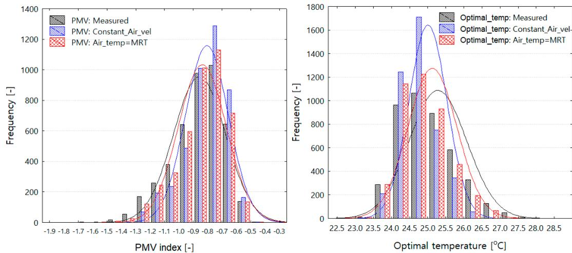
Figure 11. PMV frequency distributions in measurement and two scenarios.
