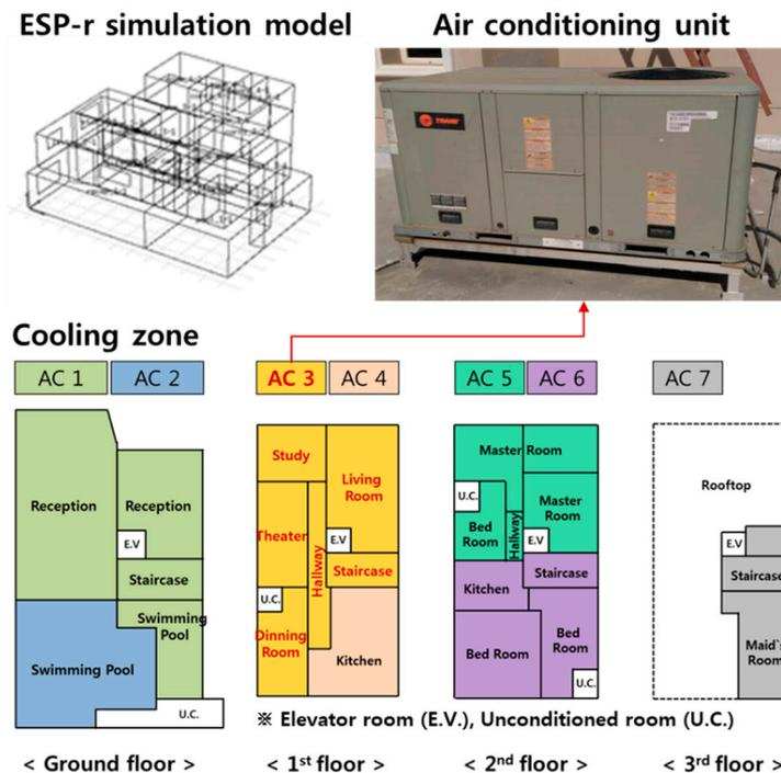
Figure 4. ESP-r simulation model and classification of cooling zones.
