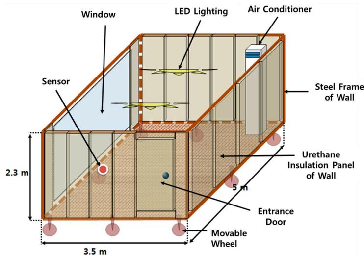
Figure 18. Size and configuration of inner chamber, location of air conditioner and sensor.
