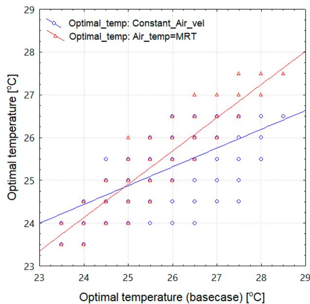
Figure 10. Optimal setpoint temperature error between the basecase and two scenarios.
