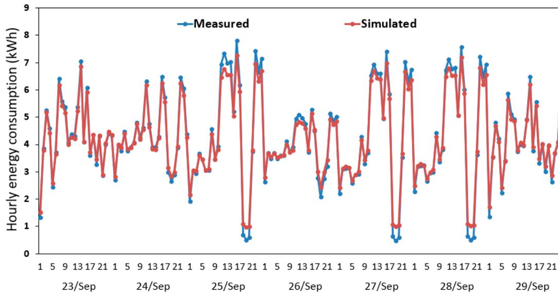
**Figure 5.** Calibration of simulation model with measurements conducted in the AC3 zone of the target house in Kuwait.
