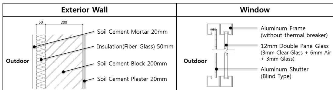
Figure 2. Exterior wall and window structures of actual houses.
