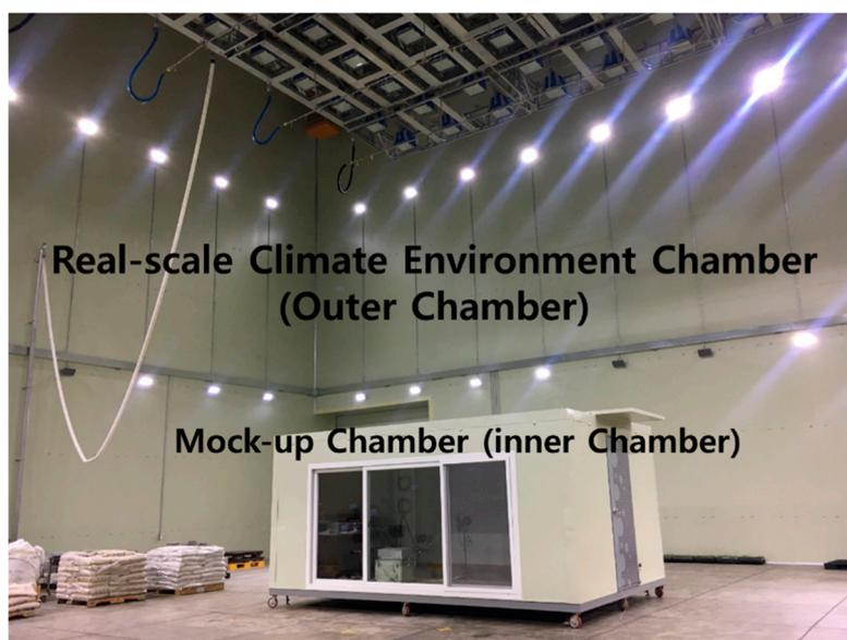
Figure 15. View of real-scale climate environment chamber and mock-up chamber for experiment.
