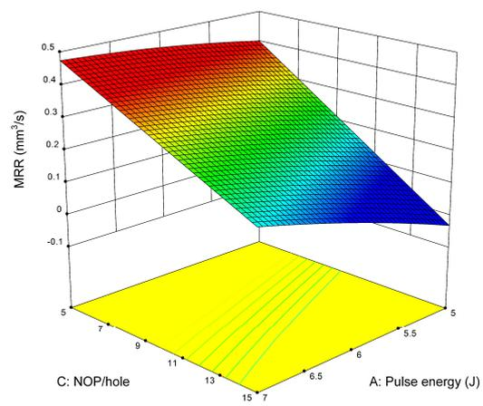
(b) Surface plot MRR vs. pulse energy and number of pulses (NOP)/hole.
