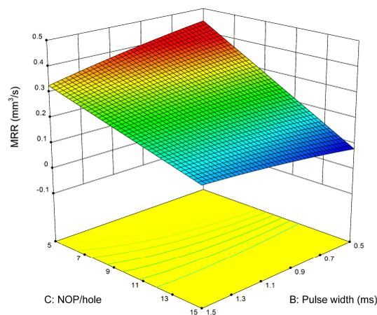
(c) Surface plot MRR vs. pulse width and NOP/hole.
