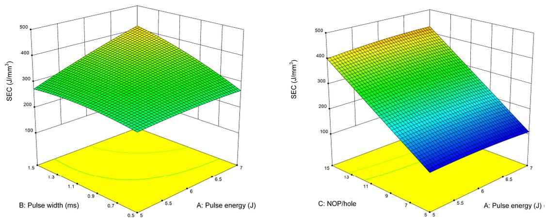
(a) Surface plot SEC vs. pulse energy and pulse width.
