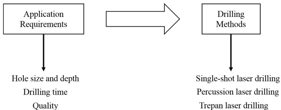
Figure 2. Laser drilling methods and the application requirements.
