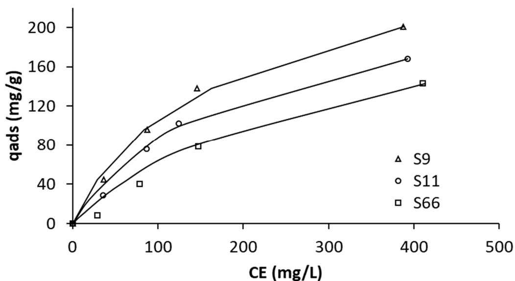
Figure S5. Asphaltenes adsorption isotherms performed for S9, S11 and S66 nanoparticles.
