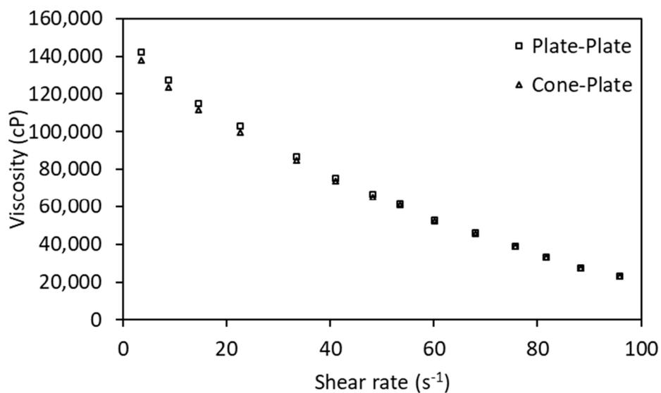
Figure S4. Rheological behavior evaluated for the EHO with a dosage of 5 vol% of xylene with plate-plate and cone-plate geometries at 30°C. .
