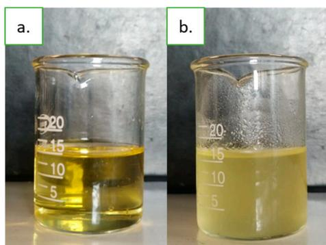
Figure S3. The visual appearance of a) the carrier fluid and b) the nanofluid. .
