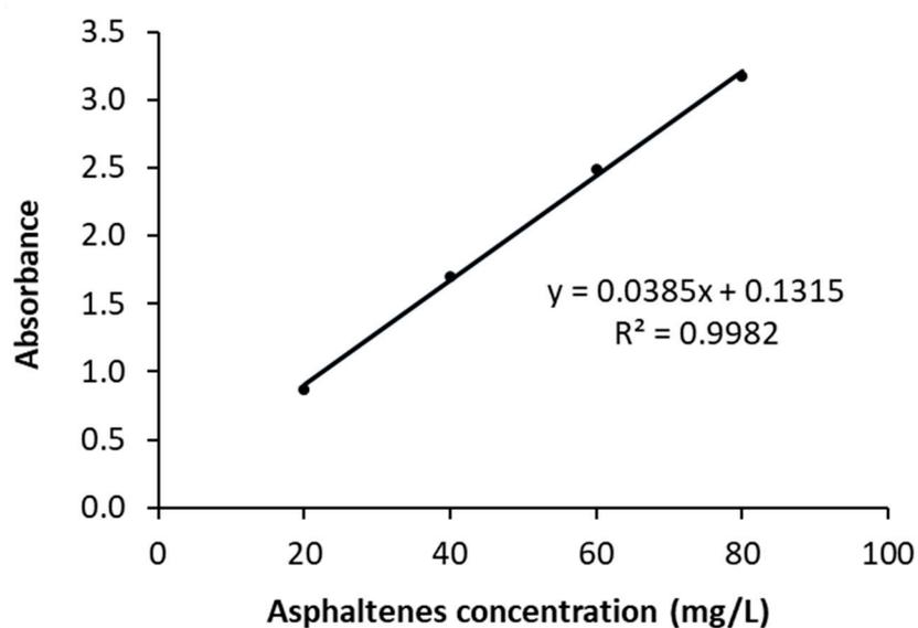
Figure S1. Calibration curve obtained for the EHO asphaltenes in toluene solutions.
