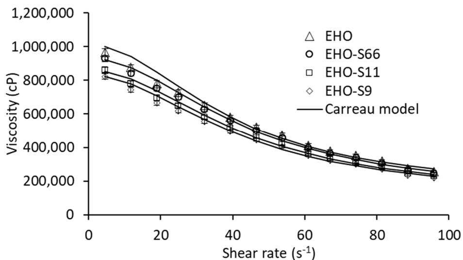
**Figure S6.** Rheological behavior of an extra-heavy oil (EHO) in the absence and presence of  $1000 \text{ mg}\cdot\text{L}^{-1}$  of  $\text{SiO}_2$  nanoparticles with different mean particle sizes of 9 (S9), 11 (S11), and 66 nm (S66) at  $30^\circ\text{C}$ . The symbols are experimental data, and the continuous lines are from the Carreau model.
