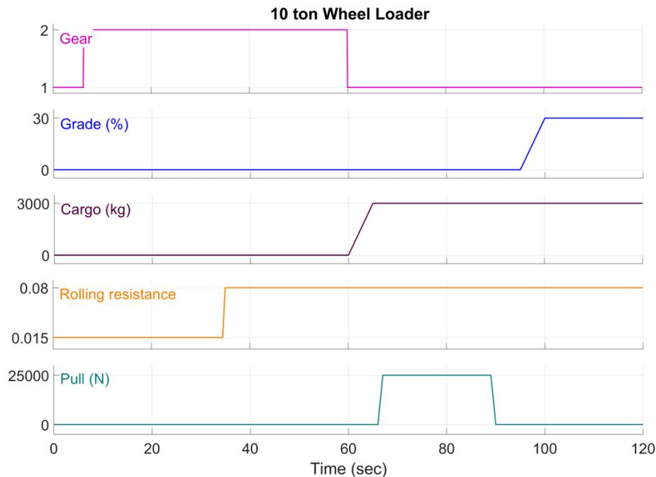
**Figure 9.** Wheel loader operation condition profiles of the predefined drive cycle.
