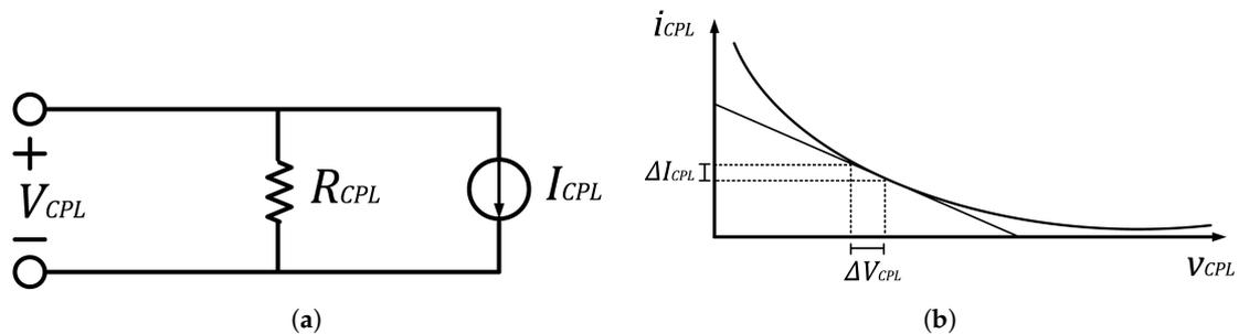
Figure 5. (a) Constant power load (CPL) simplified circuit and (b) CPL behavior curve.
