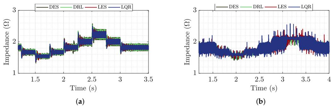
Figure 30. Impedance of the feeder buck in time during the (a) simulation and (b) test.
