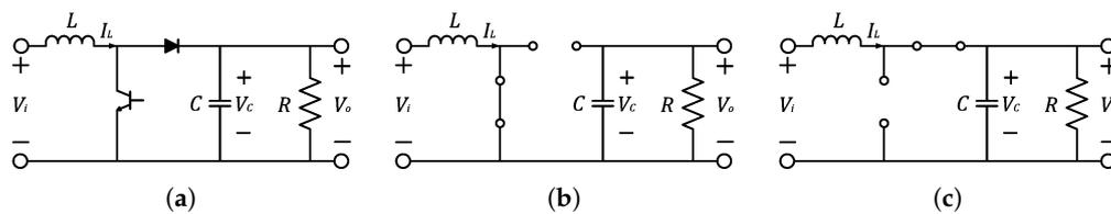
**Figure 2.** (a) Boost converter circuit. (b) Boost converter circuit for switched on condition. (c) Boost converter circuit for switched off condition.
