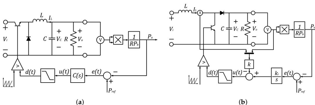
Figure 7. (a) CPL buck performed by output feedback. (b) CPL boost performed by state feedback.
