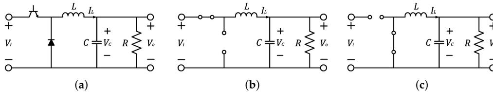
**Figure 1.** (a) Buck converter circuit. (b) Buck converter circuit for switched on condition. (c) Buck converter circuit for switched off condition.
