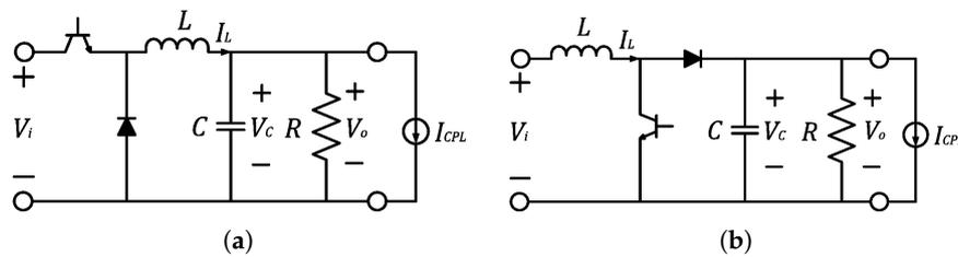
Figure 6. (a) Buck converter connected to CPL. (b) Boost converter connected to CPL.
