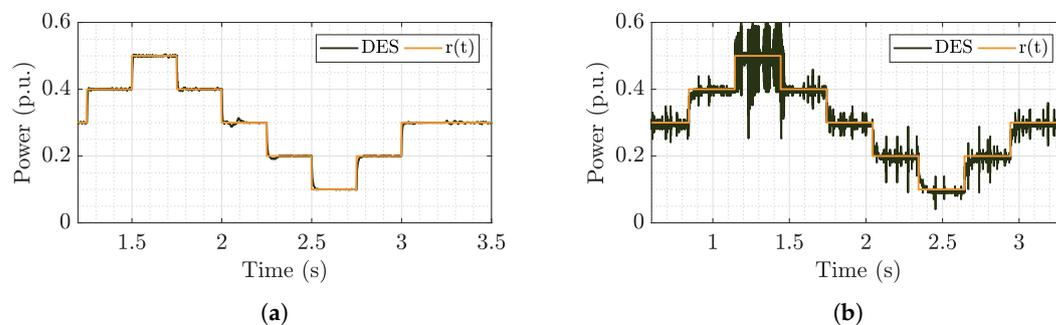
**Figure 10.** Output power for CPL buck during the (a) simulation and (b) test.
