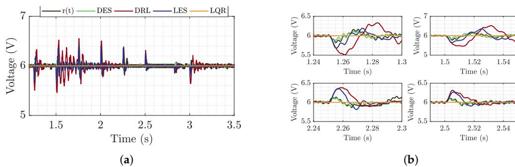
**Figure 26.** (a) Regulated voltage delivered to the DC bus. (b) Zoom to the oscillations caused by the power variation of the CPL boost during the simulation.
