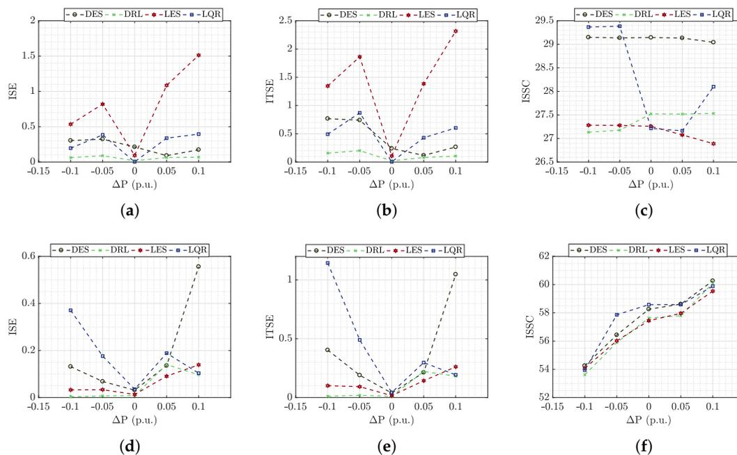
**Figure 28.** (a) ISE, (b) ITSE and (c) ISSC simulated, (d) ISE, (e) ITSE and (f) ISSC during the test for buck-boost microgrid.
