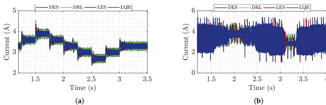
**Figure 25.** Current in the microgrid buck-boost feeder inductor during the (a) simulation and (b) test.
