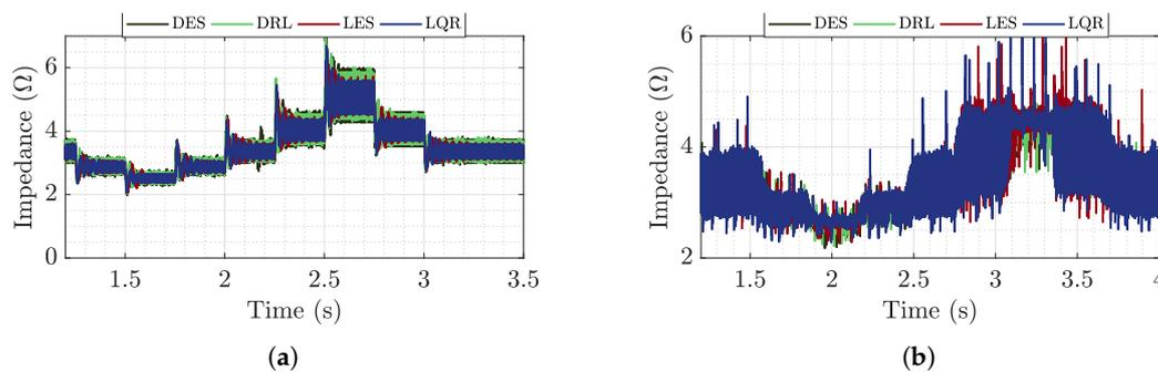
**Figure 29.** Impedance of the CPL boost in time during the (a) simulation and (b) test.
