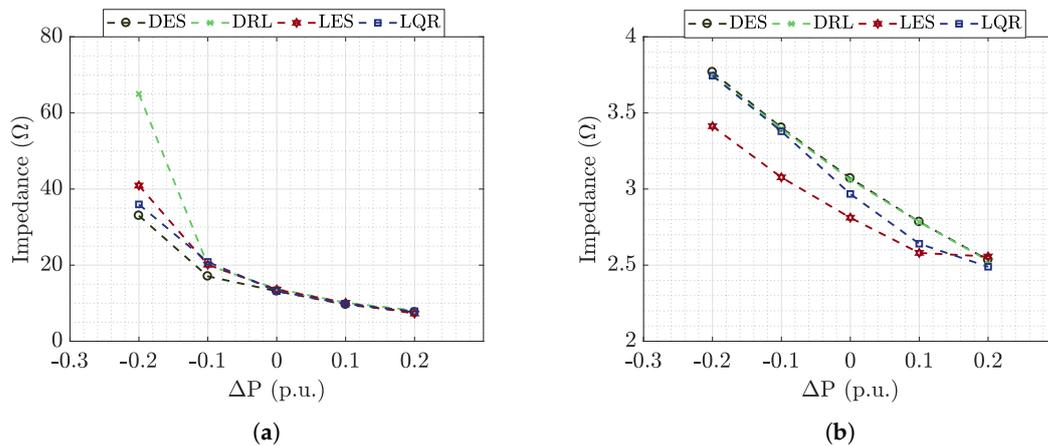
**Figure 23.** Mean CPL impedance for each power variation during the (a) simulation and (b) test.
