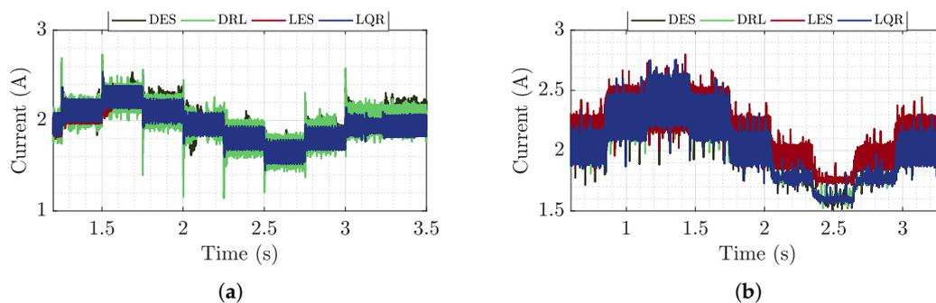
**Figure 17.** Current in the microgrid buck-buck feeder inductor during the (a) simulation and (b) test.
