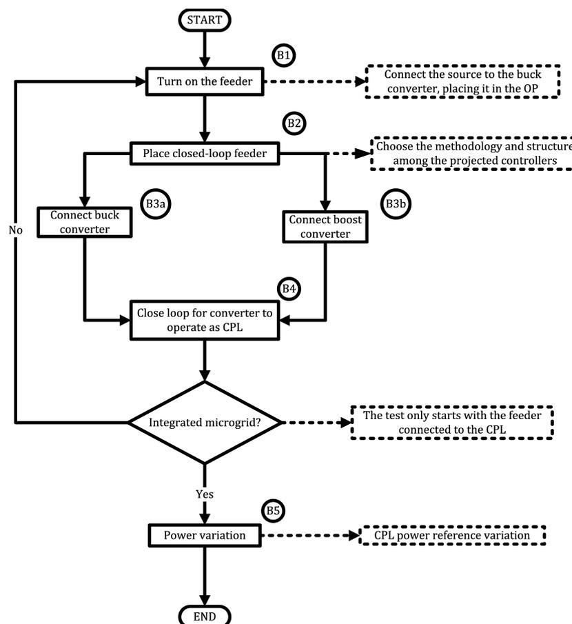
Figure 15. Flowchart of the experimental evaluation procedures.
