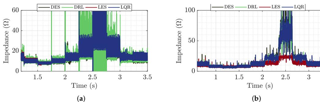
**Figure 21.** CPL buck input impedance in time during the (a) simulation and (b) test.
