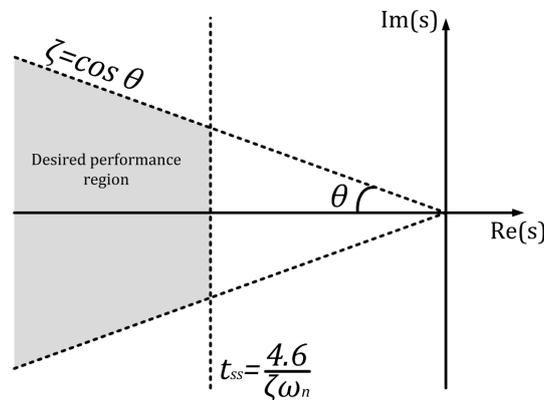
Figure 9. Desired performance region in  $s$ -plan.
