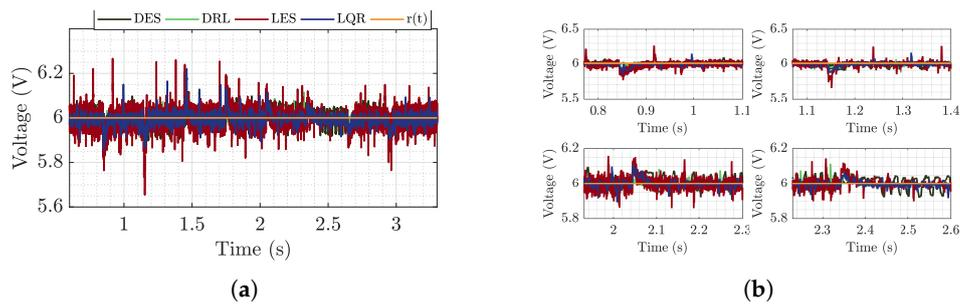
**Figure 19.** (a) Regulated voltage delivered to the DC bus during the test. (b) Zoom to the oscillations caused by the power variation of the CPL buck.
