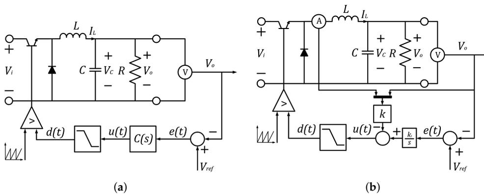
Figure 8. (a) Buck feeder using output feedback. (b) Buck feeder using state feedback with robust tracking.
