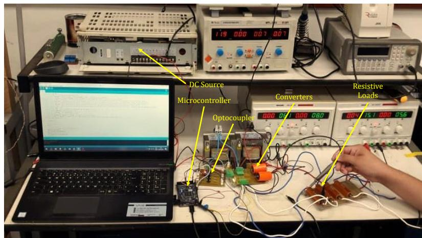
Figure 14. Experiment bench set up for testing.
