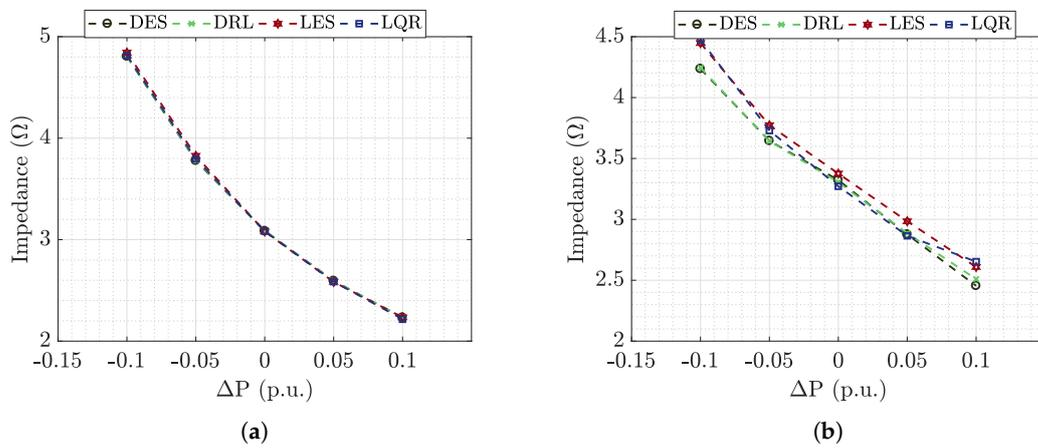
Figure 31. Mean CPL impedance for each power variation during the (a) simulation and (b) test.
