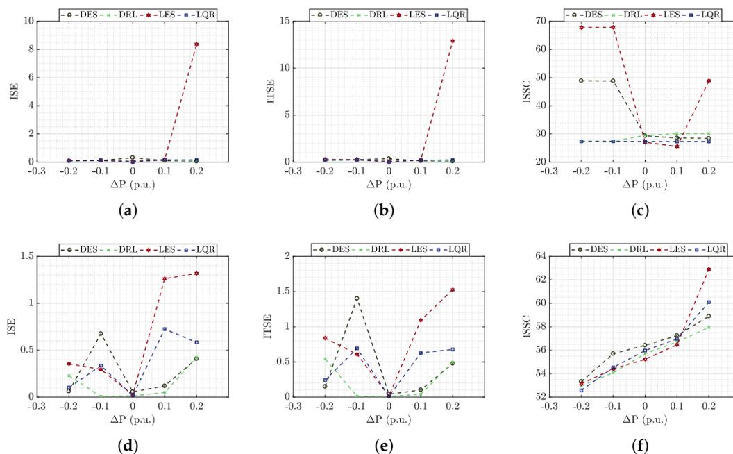
**Figure 20.** (a) Integral of squared error (ISE), (b) integral of time-weighted squared error (ITSE) and (c) integral of squared signal of control (ISSC) during the simulation, (d) ISE, (e) ITSE and (f) ISSC during the test for buck-buck microgrid.
