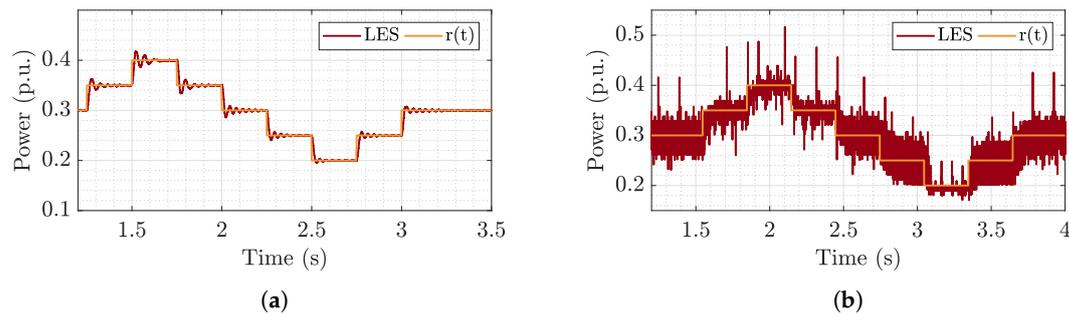
Figure 11. Output power for CPL boost during the (a) simulation and (b) test.
