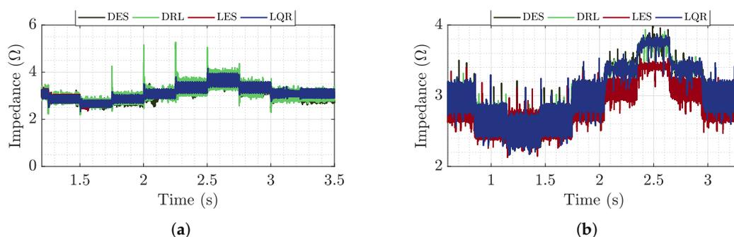
**Figure 22.** Feeder buck output impedance in time during the (a) simulation and (b) test.
