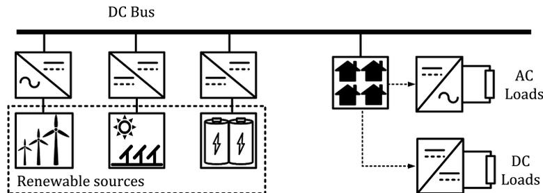
Figure 3. DC microgrid illustration.
