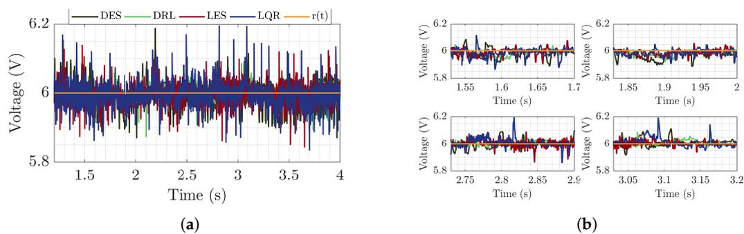
**Figure 27.** (a) Regulated voltage delivered to the DC bus. (b) Zoom to the oscillations caused by the power variation of the CPL boost during the test.
