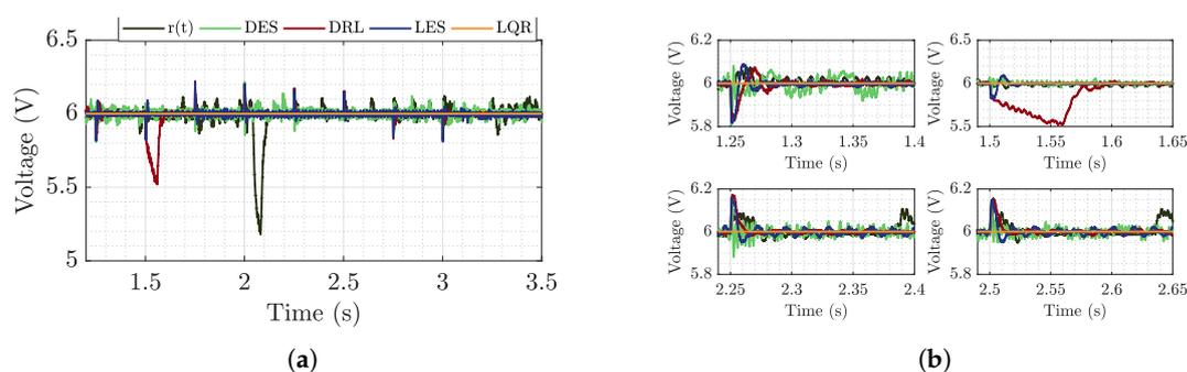
**Figure 18.** (a) Regulated voltage delivered to the DC bus during the simulation. (b) Zoom to the oscillations caused by the power variation of the CPL buck.
