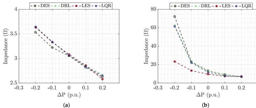
**Figure 24.** Impedance of the feeder buck in time during the (a) simulation and (b) test.
