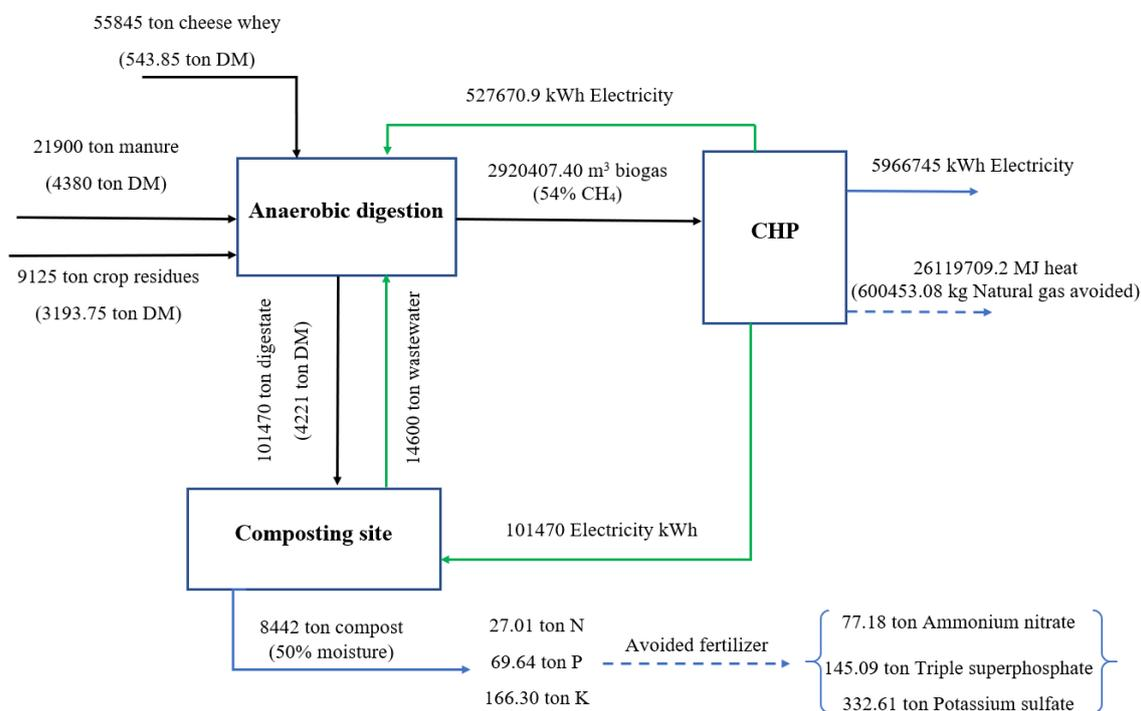
**Figure 2.** System layout and mass and energy balances referred to 1 year of operation.
