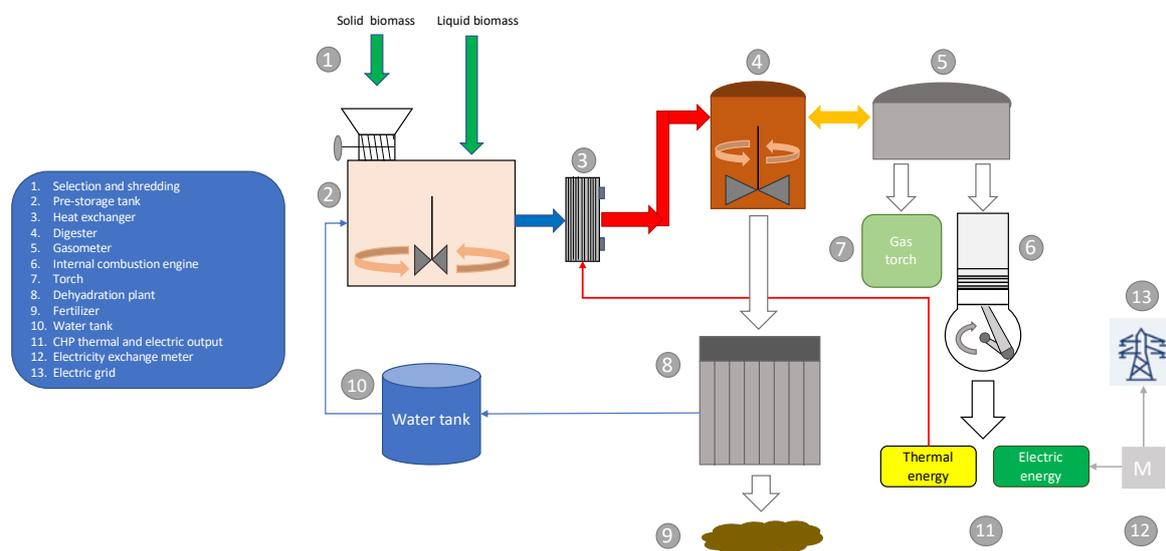
**Figure 1.** Overview of the production cycle of the plant.
