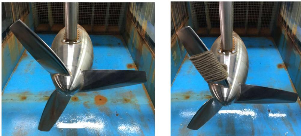
**Figure 10.** Imbalance fault (biofouling emulation) setting: healthy blade (left), imbalanced blade with 144 g attachment (right).
