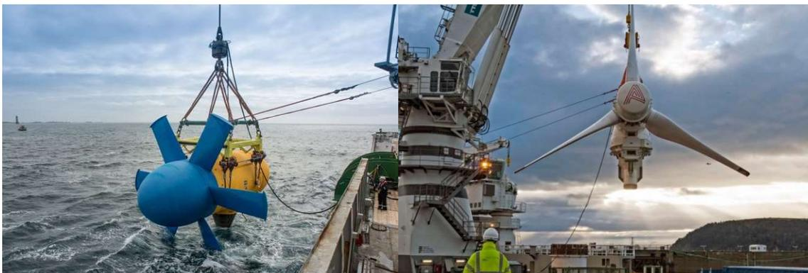
**Figure 1.** Sabella D10 (left) and Atlantis AR1500 tidal stream turbines (TSTs; right) [15].
