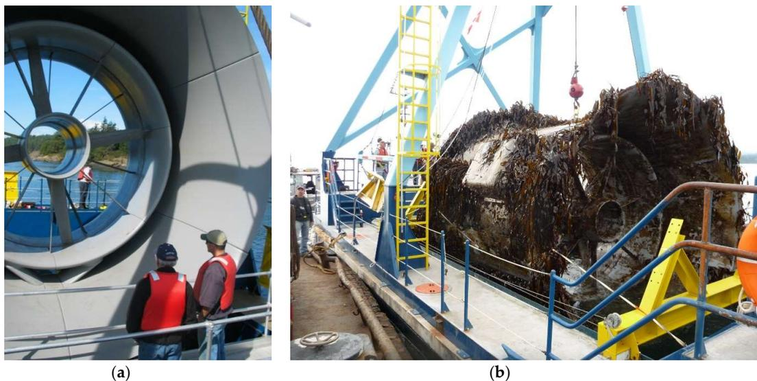
Figure 3. Biofouling attachment on a TST: (a) prior deployment, (b) TST retrieved from the ocean after some months [15,16].
