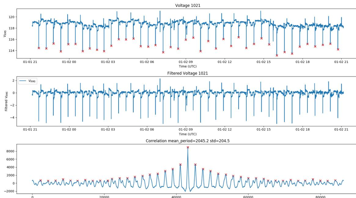
**Figure 15.** Detection of periodic voltage sags.
