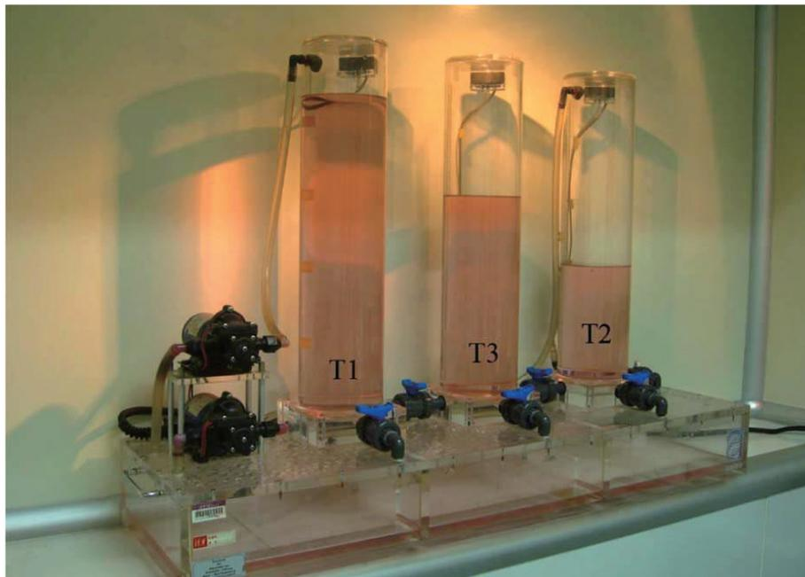
**Figure 2.** Structure of the three-tank system [33].
