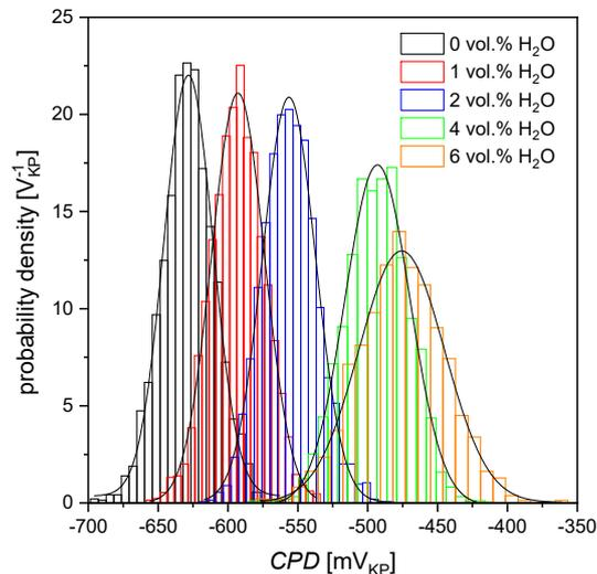
**Figure 6.** Histograms of contact potential difference (*CPD*) determined using maps shown in Figure 5; solid lines—fit of the Gaussian distribution (see Equation (7));  $V_{KP}$  is the voltage measured versus Kelvin probe.
