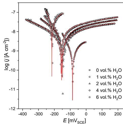
**Figure 2.** Potentiodynamic polarization curves for the AISI 1010 steel electrodes immersed in sulfolane containing up to 6 vol.% of water; symbols and solid lines represent experimental data and fit of Equation (1), respectively;  $V_{\text{SCE}}$  is the electrode potential measured vs. saturated calomel electrode.
