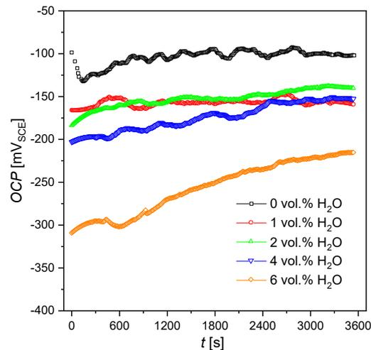
**Figure 1.** Open-circuit potential for the AISI 1010 steel electrodes immersed in sulfolane containing up to 6 vol.% of water;  $V_{\text{SCE}}$  is the electrode potential measured versus saturated calomel electrode.
