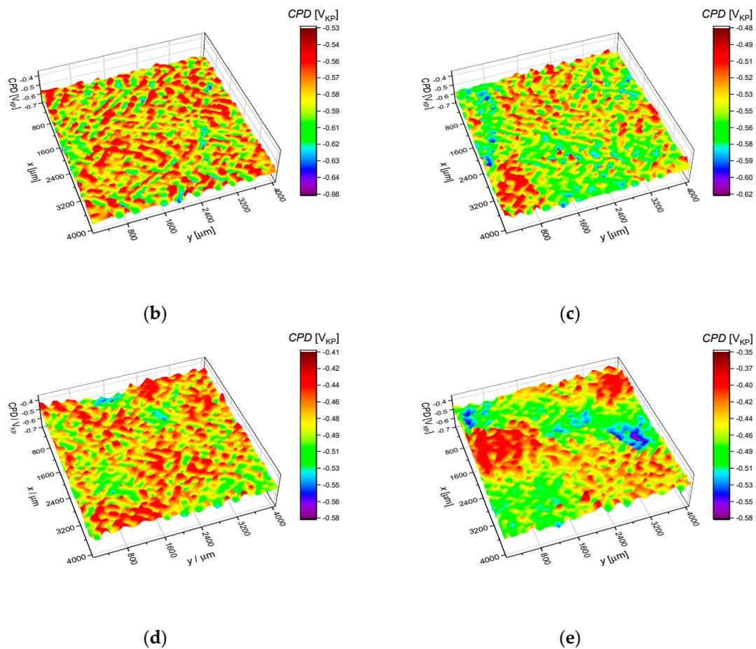
**Figure 5.** Contact potential difference (CPD) maps for the AISI 1010 steel electrodes after 96 h of immersion in sulfolane containing 0 (a), 1 (b), 2 (c), 4 (d) and 6 (e) vol.% of water;  $V_{KP}$  is the voltage measured versus Kelvin probe.
