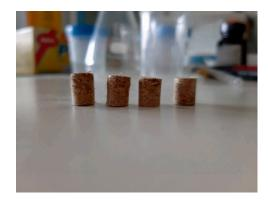
Figure 2. Pellets produced using the single press.
