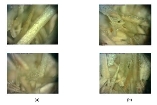
**Figure 5.** Fraction 0.3–0.85 mm (**a**) and 0.15–0.3 mm (**b**) of the straw powders at the magnification of  $50 \times$  at optical microscope.
