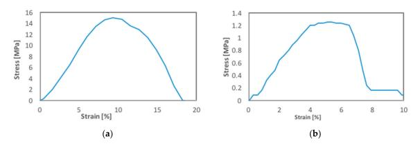
**Figure 7.** Axial compressive stress-strain curves for RS pellets (**a**) and RH pellets (**b**).
