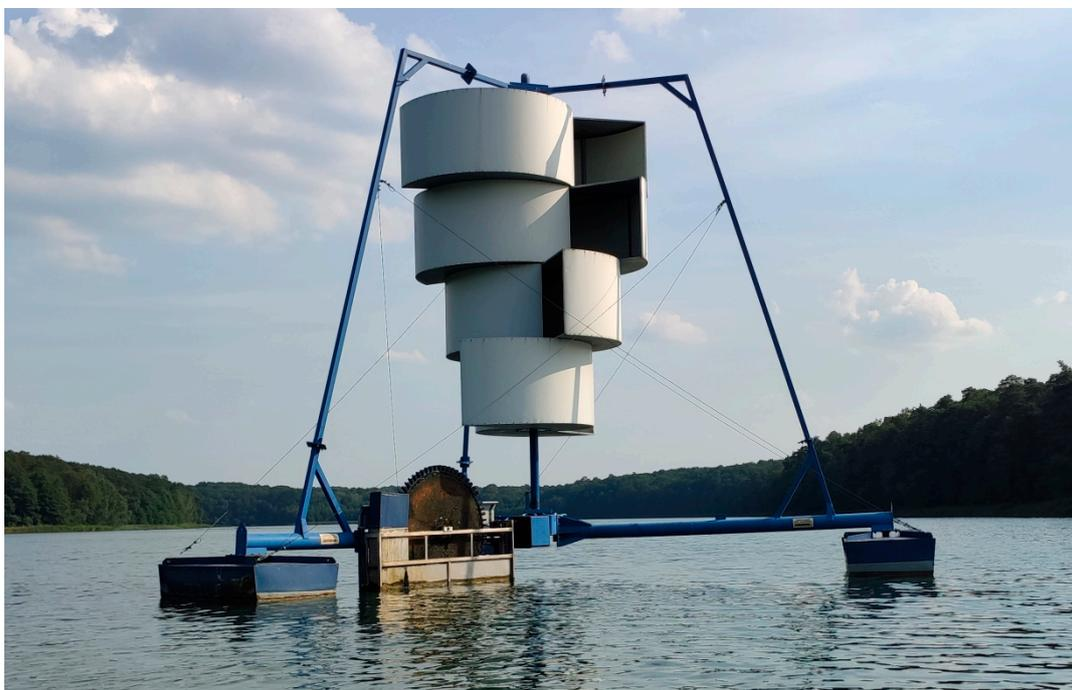
Figure 1. Wind-driven pulverizing aerator located on Góreckie Lake.
