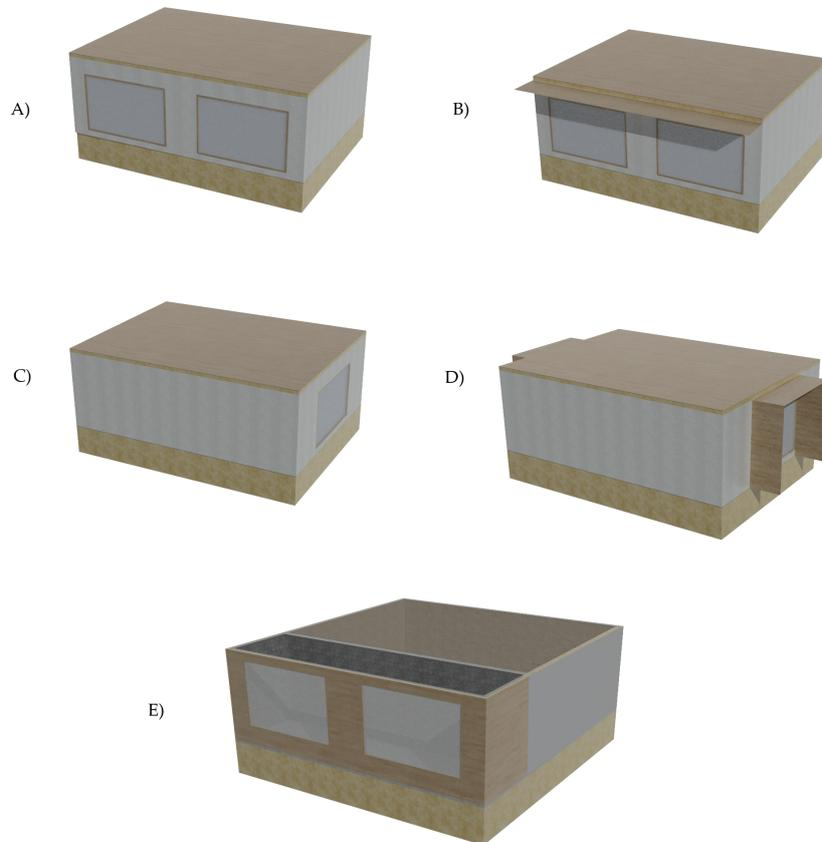
**Figure 5.** Analyzed BESTEST reference buildings: (A) Case 600, 640, 650/900, 940, 950; (B) Case 610/910; (C) Case 620/920; (D) Case 630/930; (E) Case 960.
