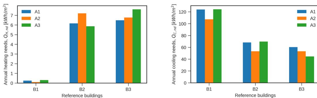
**Figure 14.** Comparison of the results described in Section 4.2.1—A1 with the results for directly downloaded weather data—A2, and the results for constructions with lower LOD—A3. The results are for littoral climate and Energy Evaluation tool.
