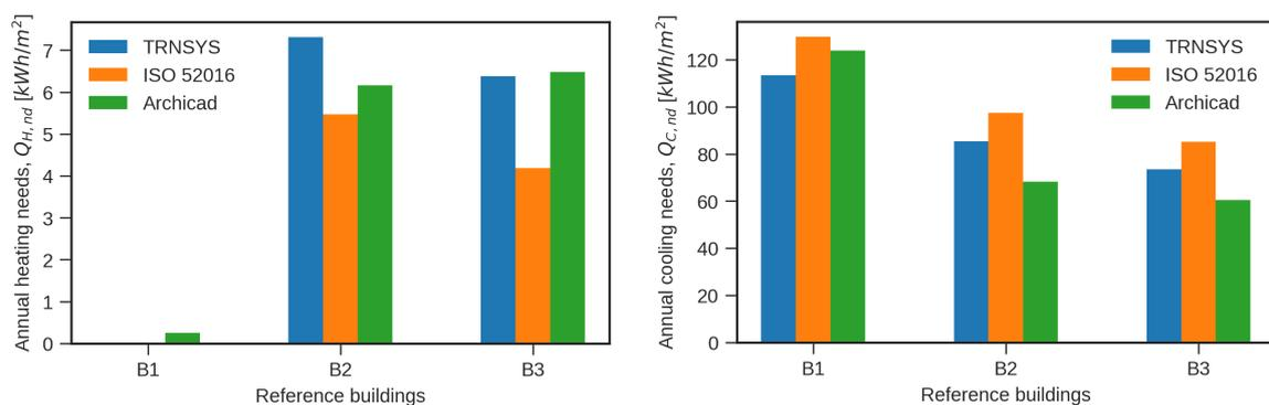
**Figure 12.** Annual heating and cooling needs for analyzed buildings in littoral climate for three types of energy simulation: TRNSYS (blue), ISO 52016-1:2017 (ISO 52016, orange), and Archicad Energy Evaluation tool (Archicad, green).
