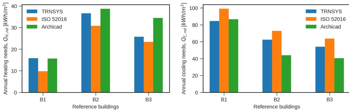
**Figure 11.** Annual heating and cooling needs for analyzed buildings in continental climate for three types of energy simulation: TRNSYS (blue), ISO 52016-1:2017 (ISO 52016, orange), and Archicad Energy Evaluation tool (Archicad, green).
