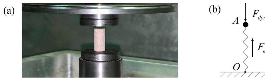
**Figure 5.** The “mass-on-a-spring” model: (a) a sample in the set-up; (b) schematics of the model.
