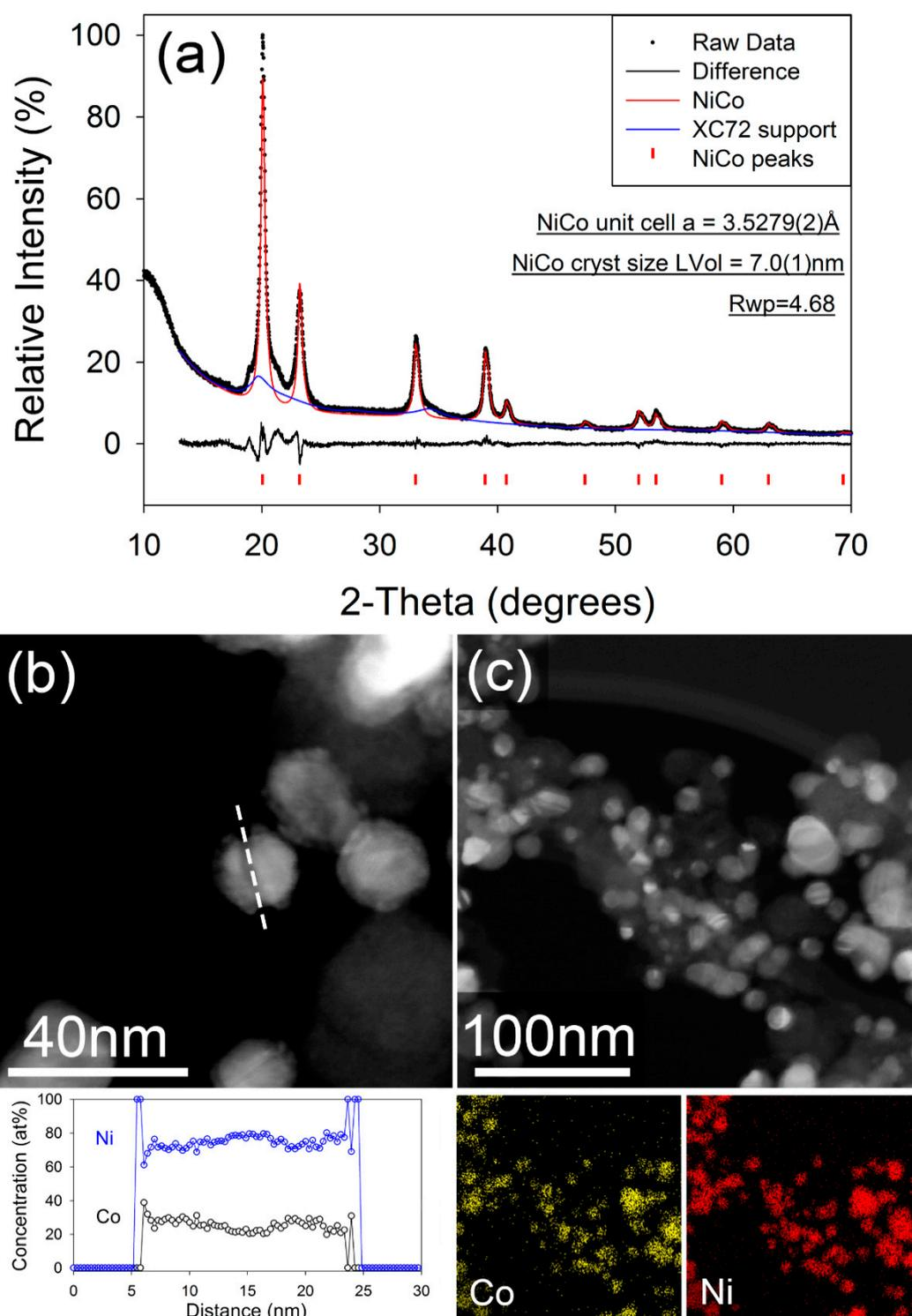
**Figure 5.** (a) Fitted X-ray diffraction pattern for NiCo/C after annealing. Data were collected in capillary transmission mode using a Mo- $K_{\alpha}$  source and modelled using a Rietveld-type approach. (b) Dark field image of annealed NiCo/C nanoparticles, with composition measured along the dashed line. (c) Dark field STEM image of annealed NiCo/C nanoparticles with corresponding X-ray element maps of Co (yellow), and Ni (red).
