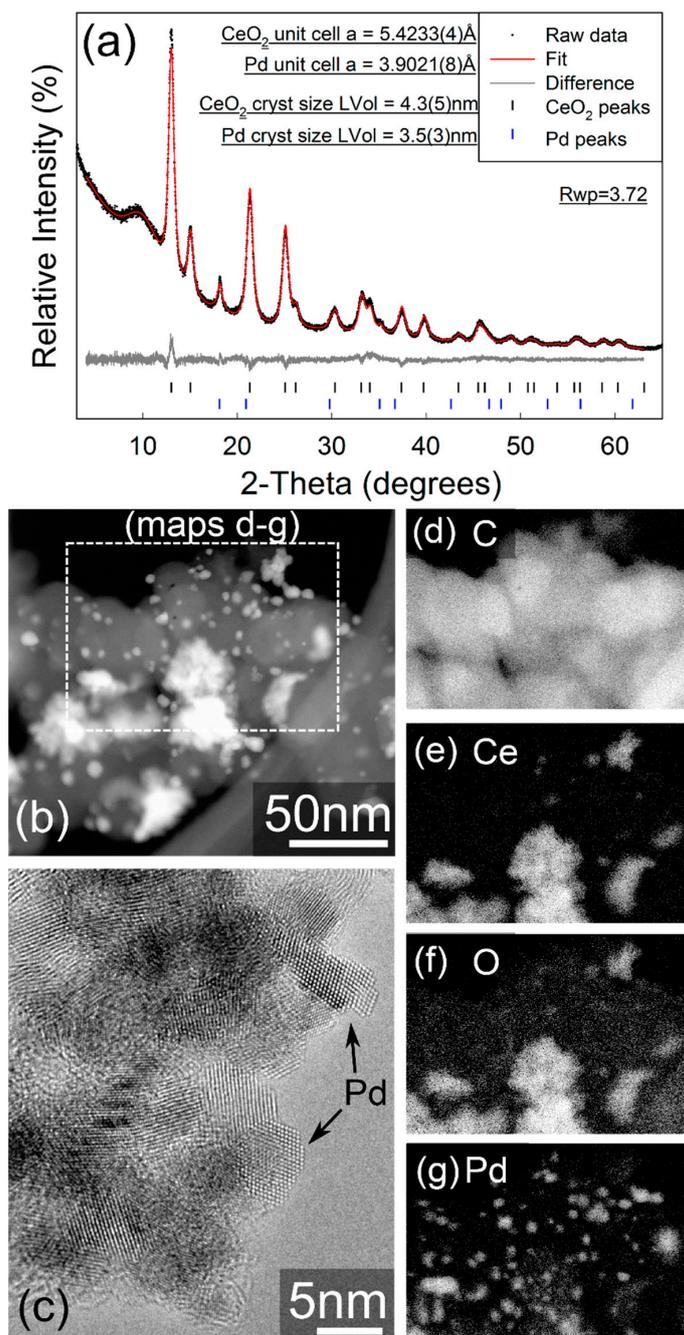
**Figure 2.** (a) Fitted X-ray powder diffractogram for Pd/C-CeO<sub>2</sub>. Data were collected in capillary transmission mode using a Mo-K<sub>α</sub> source and modelled using a Rietveld-type approach. The “amorphous bump” at approx. 9° 2θ is due to the Kapton capillary material. (b) Annular dark-field STEM image, (c) high-resolution TEM image showing crystalline Pd particles, (d–g) elemental EDX images acquired within the area indicated in (b). Gamma adjustments were applied in (b,d–g).
