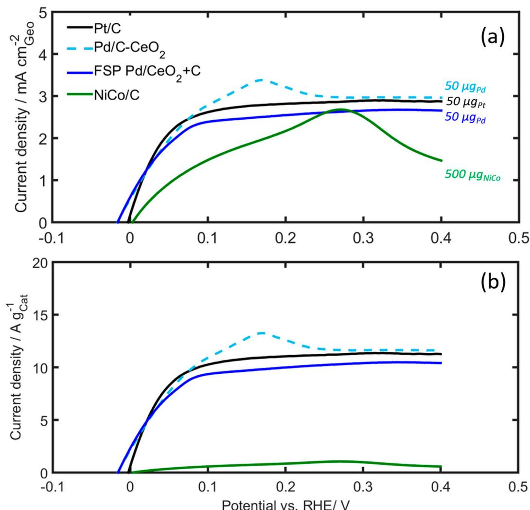
**Figure 7.** RDE voltammograms of Pd/C-CeO<sub>2</sub>, Pd/CeO<sub>2</sub> + C and NiCo/C compared to Pt/C in H<sub>2</sub>-saturated 0.1 M KOH. (a) Geometric current density, and (b) mass specific current density. Scan rate: 5 mV/s, rotating speed: 1600 rpm. The catalyst loading was 500 µg based on NiCo, and 50 µg for the PGM catalysts.
