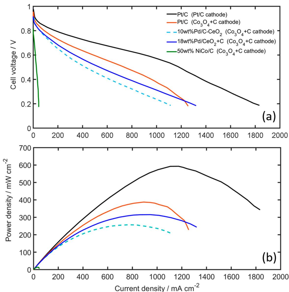
**Figure 8.** (a) Polarization, and (b) power density curves of the AEMFC using various anode and cathode catalysts (cathodes are denoted within parenthesis in the legend). Measurements taken at 70 °C, H<sub>2</sub> and O<sub>2</sub> on anode and cathode, using 1.0 and 0.5 slpm, respectively. Gas dew points are 68 and 73 °C for the anode and cathode, respectively.
