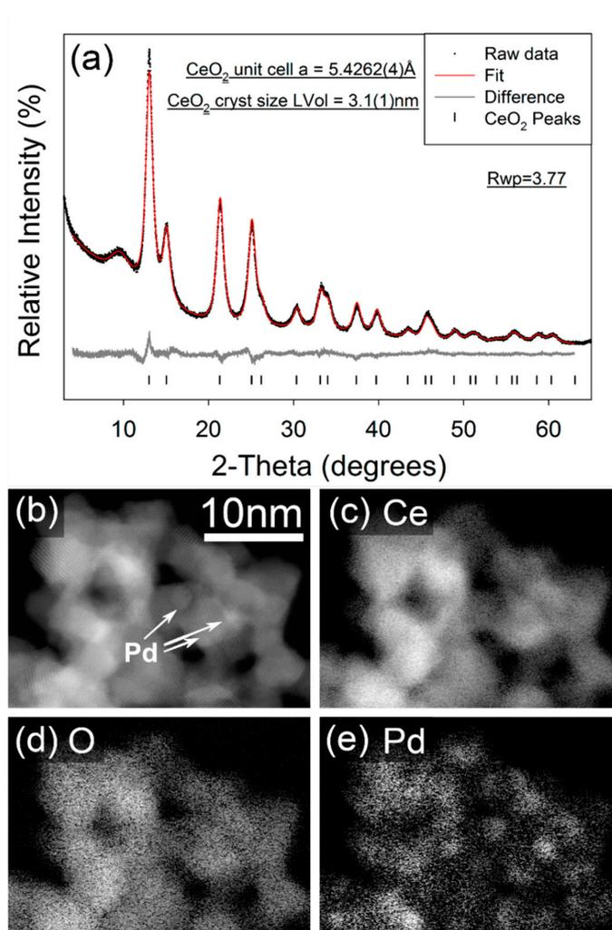
**Figure 3.** (a) Fitted X-ray powder diffractograms for FSP synthesized FSP Pd/CeO<sub>2</sub>. Data were collected in capillary transmission mode using a Mo-K<sub>α</sub> source and modelled using a Rietveld-type approach. The “amorphous bump” at ~9° 2-Theta is due to the Kapton capillary material, (b) STEM image, and (c–e) elemental EELS maps from FSP Pd/CeO<sub>2</sub>.
