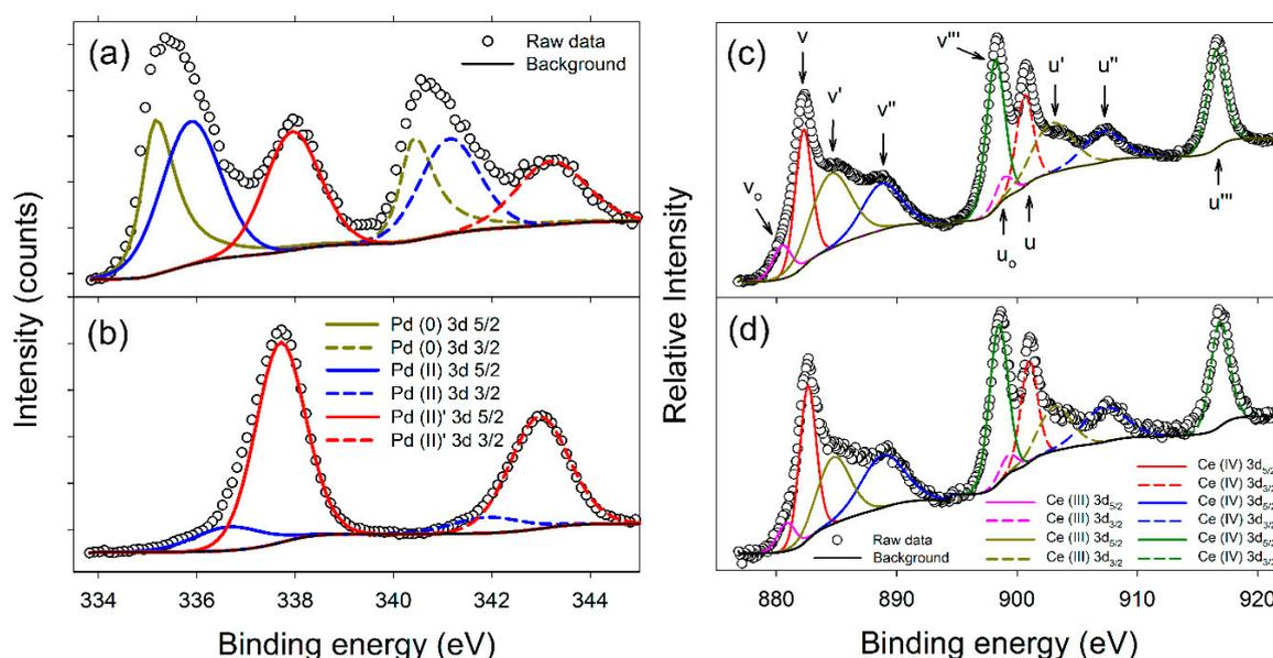
**Figure 4.** XPS data for Pd for (a) Pd/C-CeO<sub>2</sub>, and (b) FSP Pd/CeO<sub>2</sub>. Lines marked Pd(0), Pd(II) and Pd(II) are assigned respectively to metallic Pd, sub-stoichiometric PdO and super-stoichiometric PdO. XPS data for Ce for (c) Pd/C-CeO<sub>2</sub>, and (d) FSP Pd/CeO<sub>2</sub>. To aid comparison with previous work, the commonly used nomenclature of Burroughs et al. [30] was adopted in (c).
