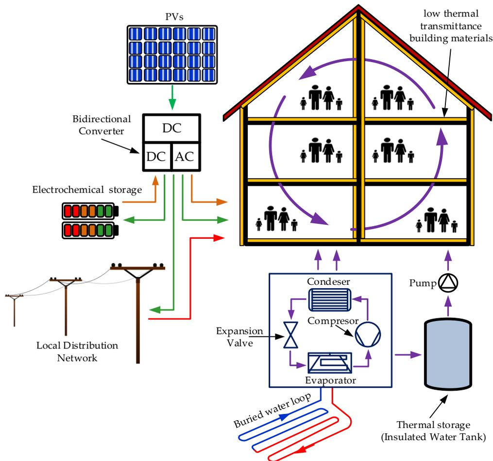
**Figure 1.** Schematic diagram of the proposed nZEB concept.
