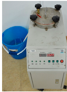
Figure 2. Saturated water test machine.
