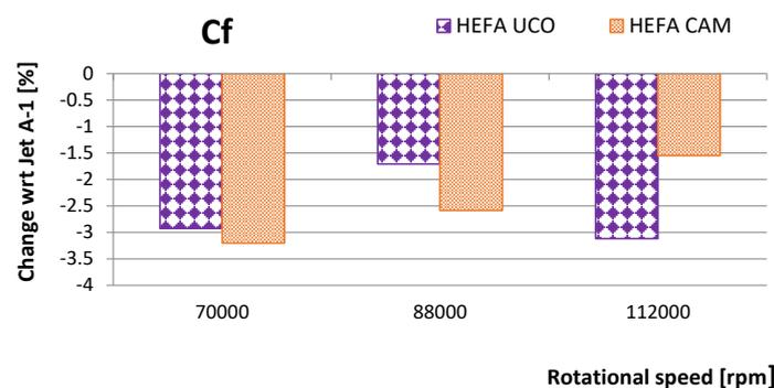
**Figure 4.** Changes of fuel consumption for synthetic blending components with regard to Jet A-1.
