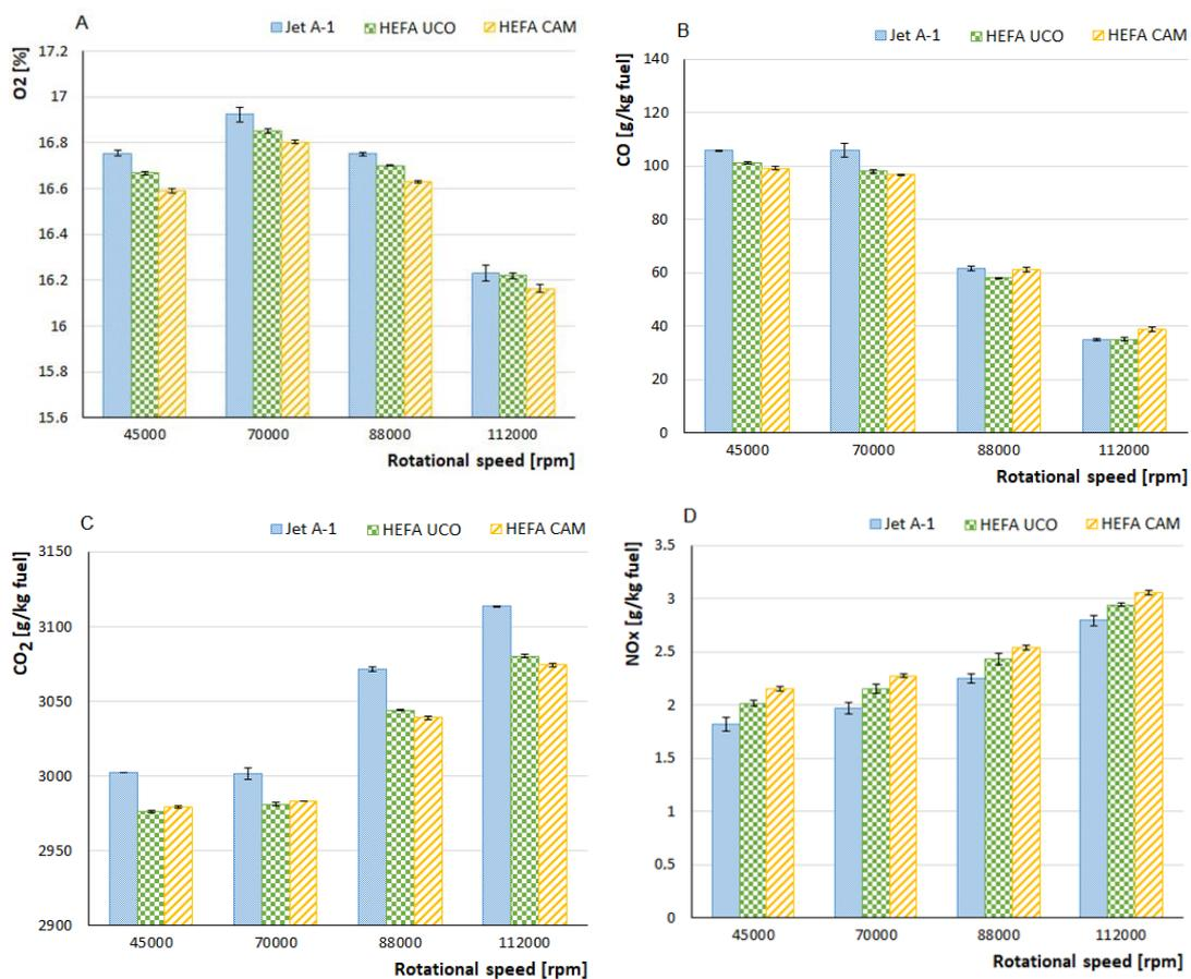
Figure 6. Selected gas component emission as a function of rotational speed. (A) O<sub>2</sub>, (B) EI CO, (C) EI CO<sub>2</sub>, (D) EI NO<sub>x</sub>.
