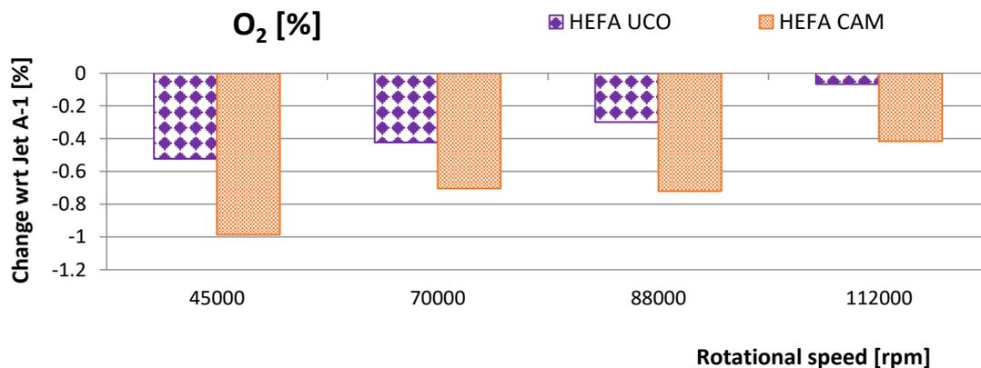
Figure 7. Changes of O<sub>2</sub> emission for synthetic blending components with regard to Jet A-1.
