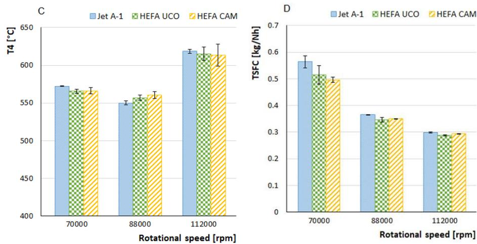
**Figure 2.** Selected engine parameters as a function of rotational speed. (A) thrust, (B) fuel consumption, (C) turbine temperature, (D) thrust specific fuel consumptions.
