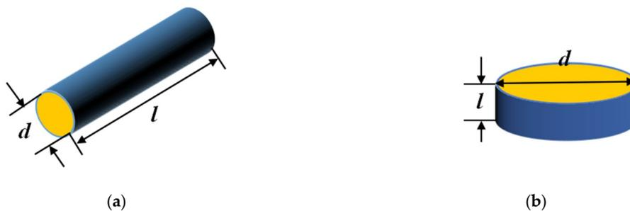
**Figure 1.** Geometries of (a) a rod and (b) a disk modeled in the present DEM simulations.
