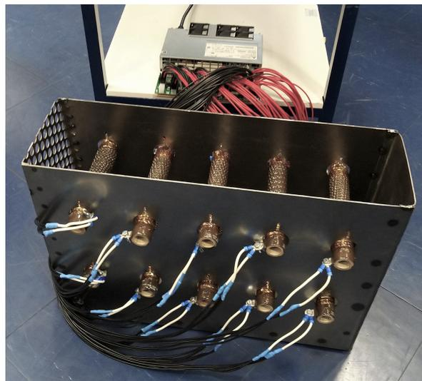
Figure 8. Modular passive load for emulating DC power consumption.
