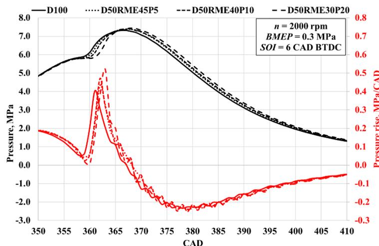
**Figure 6.** Dependence of pressure and pressure rise in the cylinder on the crank angle degree.
