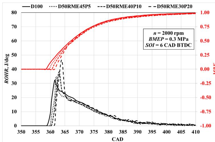
**Figure 7.** Dependence of the rate of heat release and the mass burnt fraction on the crank angle degree.
