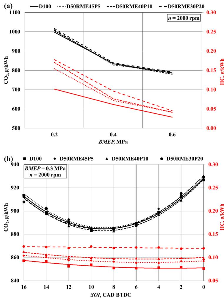
**Figure 4.** Dependence of carbon dioxide emissions and hydrocarbons on different: (a) loads; (b) injection timing.
