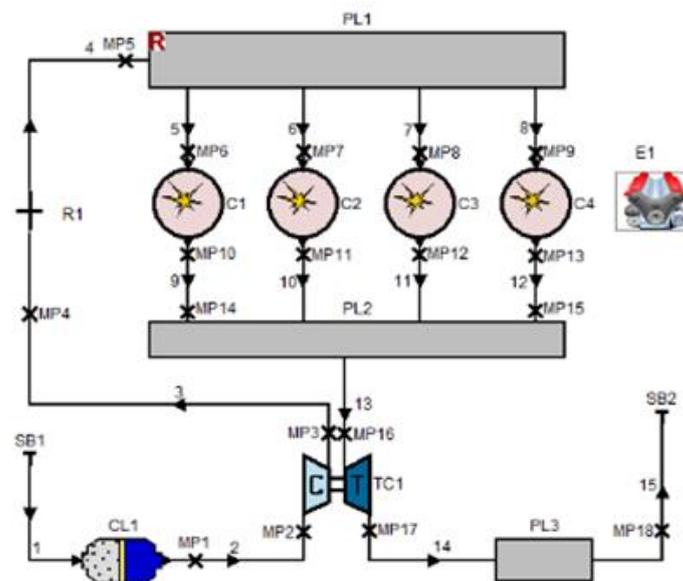
Figure 2. Digital Engine Model used in AVL BOOST.
