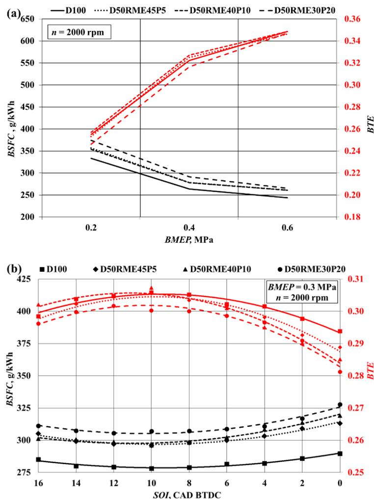
**Figure 3.** Dependence of Brake Specific Fuel Consumption and Brake Thermal Efficiency on different: (a) loads; (b) injection timing.
