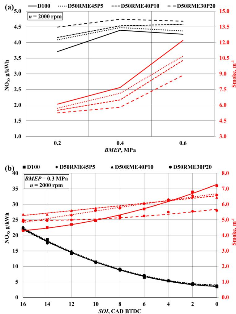
Figure 5. Dependence of nitrogen oxide emissions and smoke on different: (a) loads; (b) injection timing.
