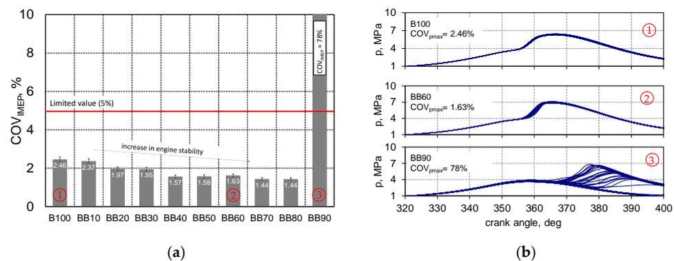
Figure 7. COV of IMEP (a) and cycle-by-cycle variation (b).
