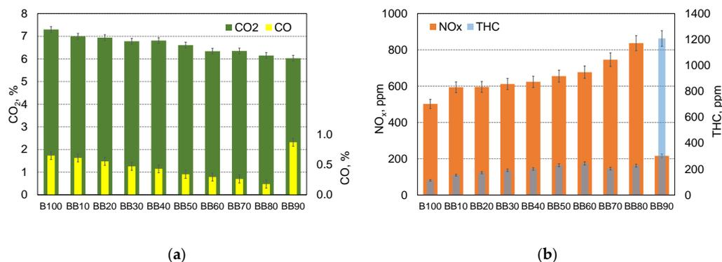
**Figure 11.** Engine exhaust emissions CO and CO<sub>2</sub> (a) and NO<sub>x</sub> and THC (b).
