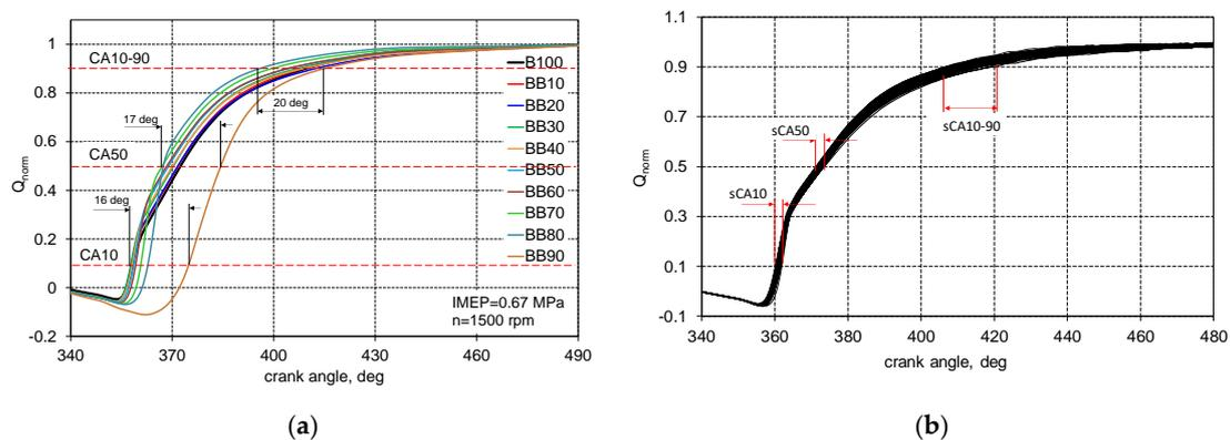
**Figure 9.** Normalized heat release and combustion stages (a) and the spread of the characteristic stages of combustion (b).
