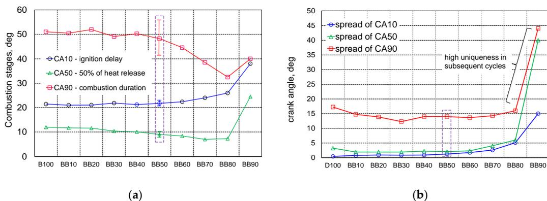
**Figure 10.** Combustion stages (a) and spread of combustion stages (b).
