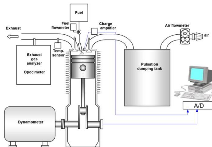
Figure 1. Diagram of the test stand.
