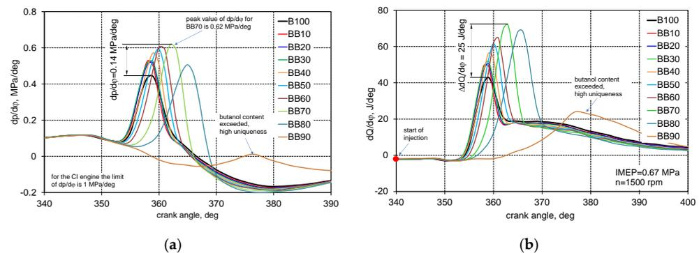
**Figure 5.** Pressure increase rate (a) and heat release rate (b).
