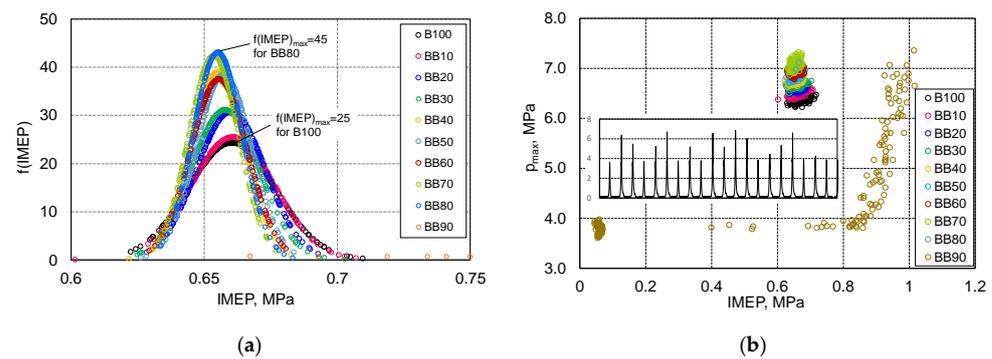
**Figure 8.** Probability density of indicated mean effective pressure (a) and relationship between IMEP and  $p_{\max}$  (b).
