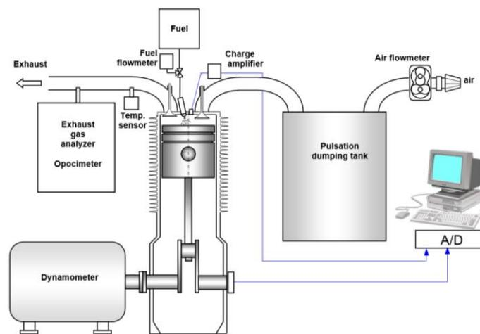
Figure 1. Diagram of the test stand.
