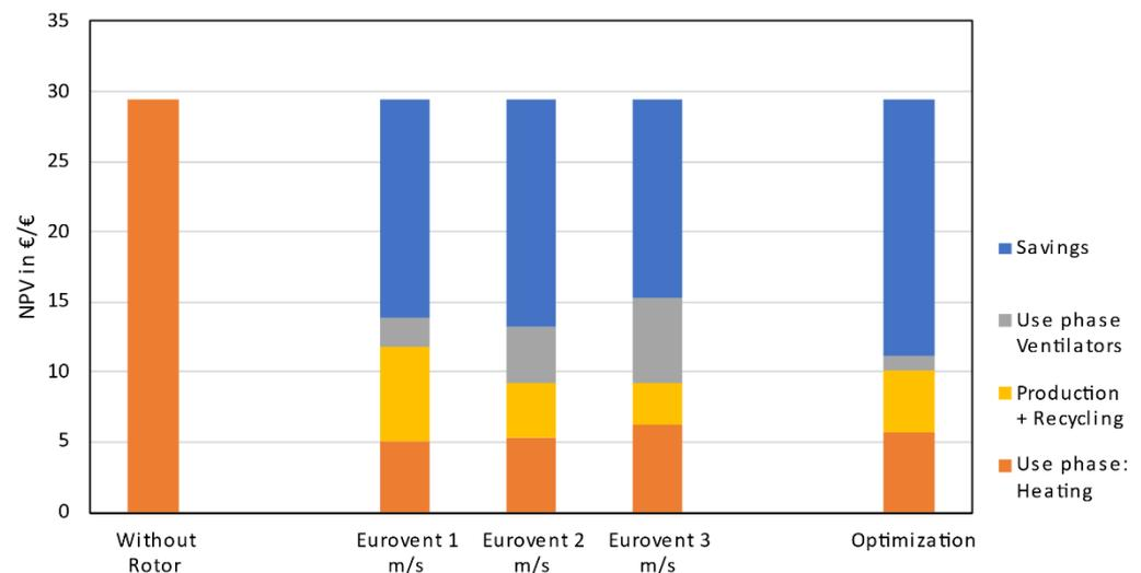
**Figure 9.** 25 €/t CO<sub>2</sub> Eq. scenario with optimized RHX and Eurovent RHX under different operating ambient air empty tube velocities at 10,000 m<sup>3</sup>/h.
