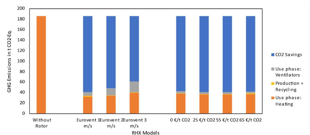
**Figure 5.** Total life cycle GHG emissions in CO<sub>2</sub> Eq. for different optimized RHXs and the Eurovent model at an FU of 10,000 m<sup>3</sup>/h.
