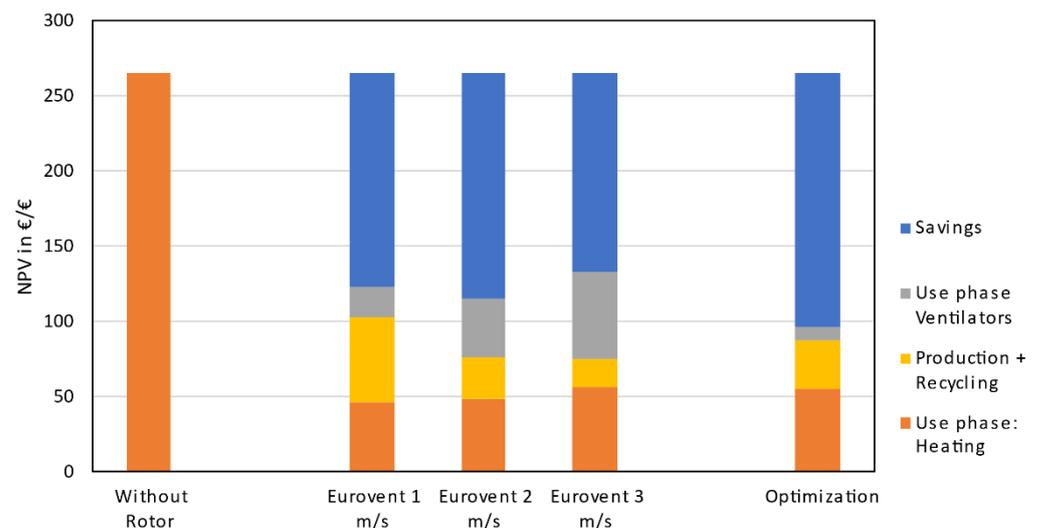
**Figure 8.** Scenario 0 €/t CO<sub>2</sub> Eq. with optimized RHX and Eurovent RHX under different operating ambient air empty tube velocities at 100,000 m<sup>3</sup>/h.
