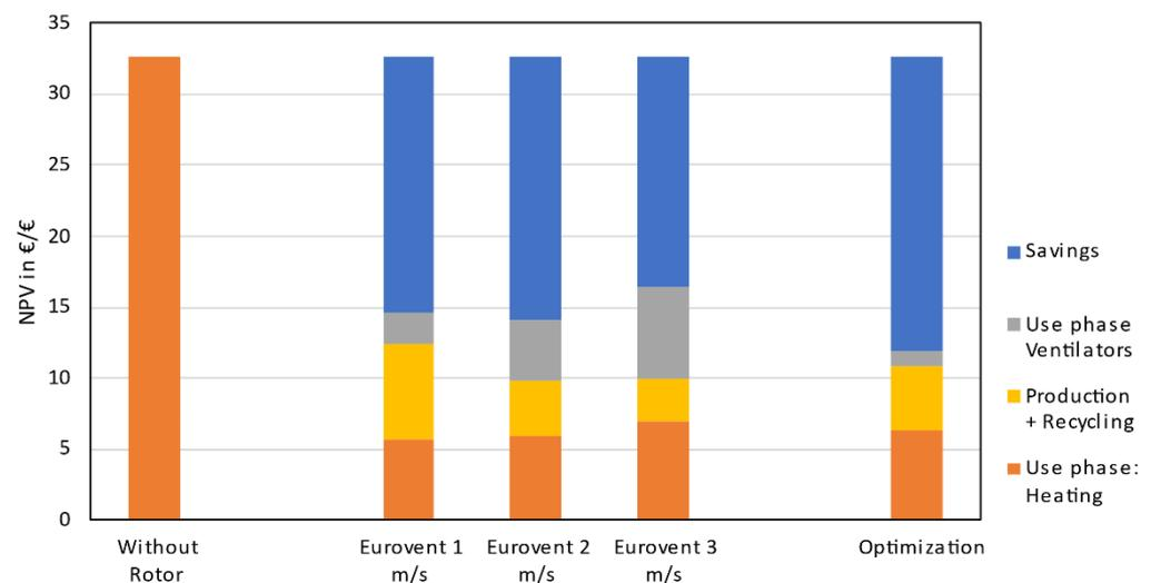
**Figure 10.** 55 €/t CO<sub>2</sub> Eq. scenario with optimized RHX and Eurovent RHX under different operating ambient air empty tube velocities at 10,000 m<sup>3</sup>/h.
