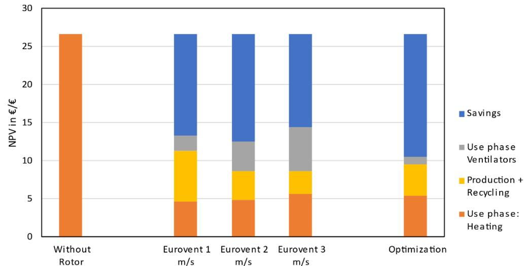
**Figure 7.** Scenario 0 €/t CO<sub>2</sub> Eq. with optimized RHX and Eurovent RHX under different operating ambient air empty tube velocities at 10,000 m<sup>3</sup>/h.
