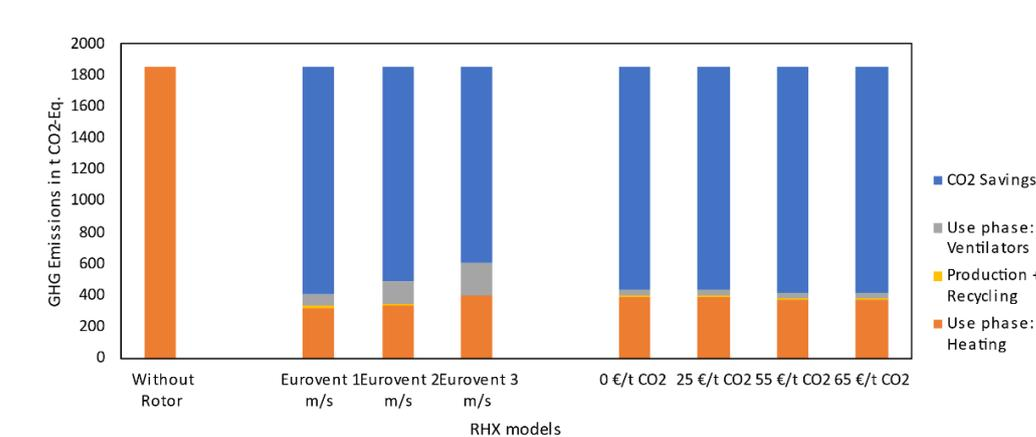
**Figure 6.** Total life cycle GHG emissions in CO<sub>2</sub> Eq. for different optimized RHXs and the Eurovent model at an FU of 100,000 m<sup>3</sup>/h.
