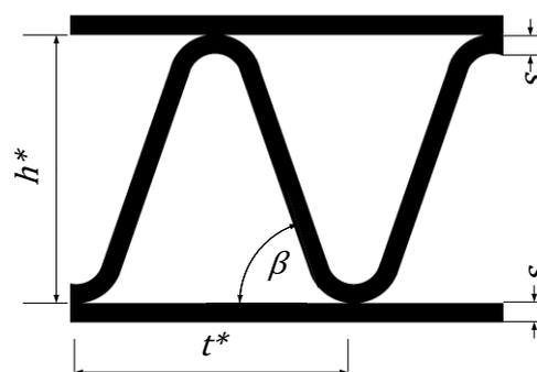
Figure 2. RHX cross-section.
