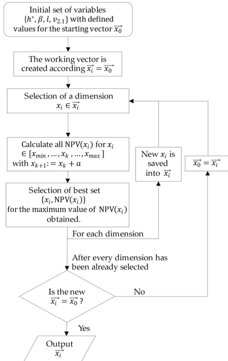
Figure 4. Optimization algorithm flow diagram.
