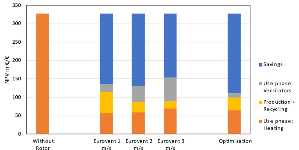
**Figure A3.** 55 €/t CO<sub>2</sub> Eq. scenario with optimized RHX and Eurovent RHX under different operating ambient air empty tube velocities at 100,000 m<sup>3</sup>/h.
