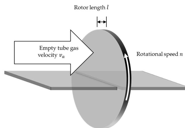
**Figure 3.** RHX length  $l$  and operational parameters.
