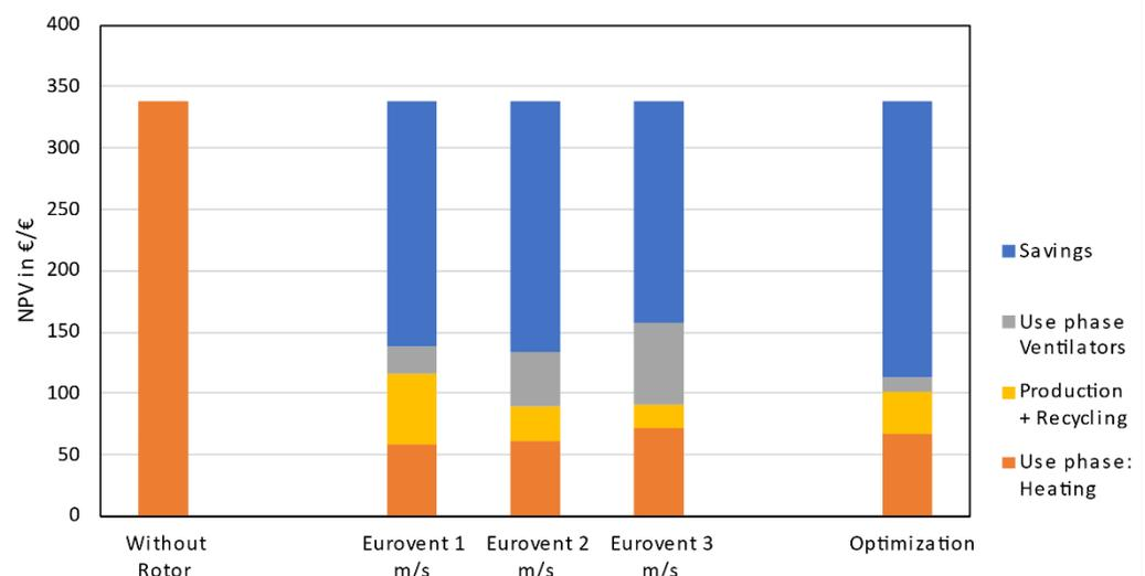
**Figure A4.** 65 €/t CO<sub>2</sub> Eq. scenario with optimized RHX and Eurovent RHX under different operating ambient air empty tube velocities at 100,000 m<sup>3</sup>/h.
