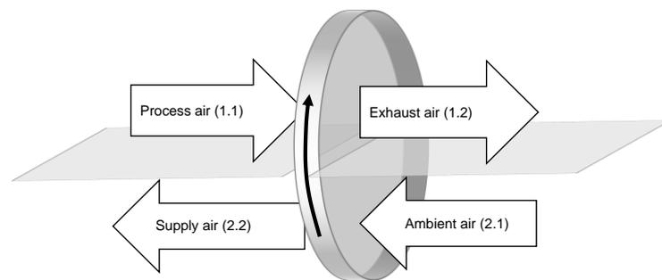
**Figure 1.** RHX working principle and stream names.
