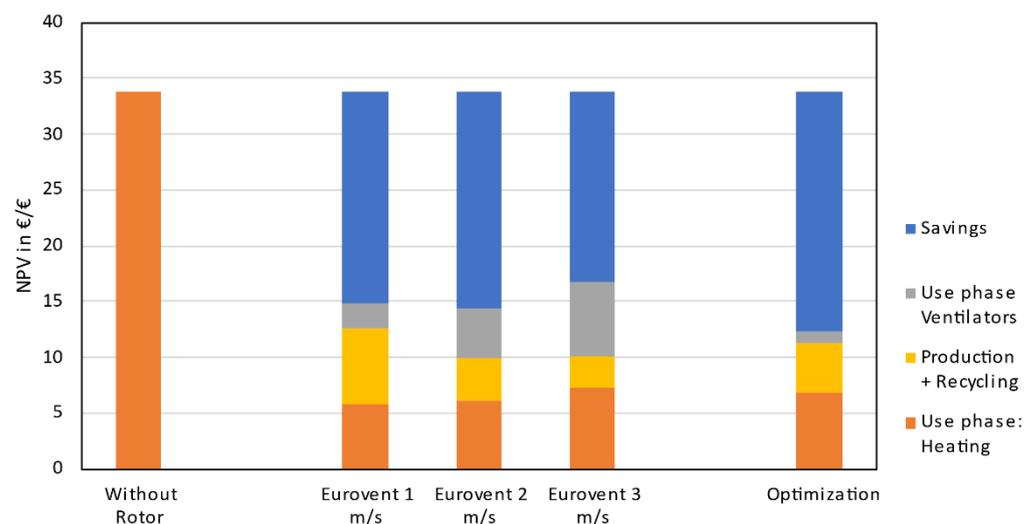
**Figure 11.** 65 €/t CO<sub>2</sub> Eq. scenario with optimized RHX and Eurovent RHX under different operating ambient air empty tube velocities at 10,000 m<sup>3</sup>/h.
