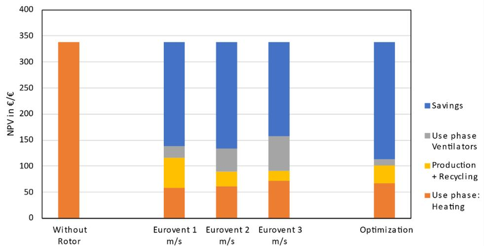
**Figure A1.** 65 €/t  $\text{CO}_2$  Eq. scenario with optimized RHX and Eurovent RHX under different operating ambient air empty tube velocities at  $100,000 \text{ m}^3/\text{h}$ .
