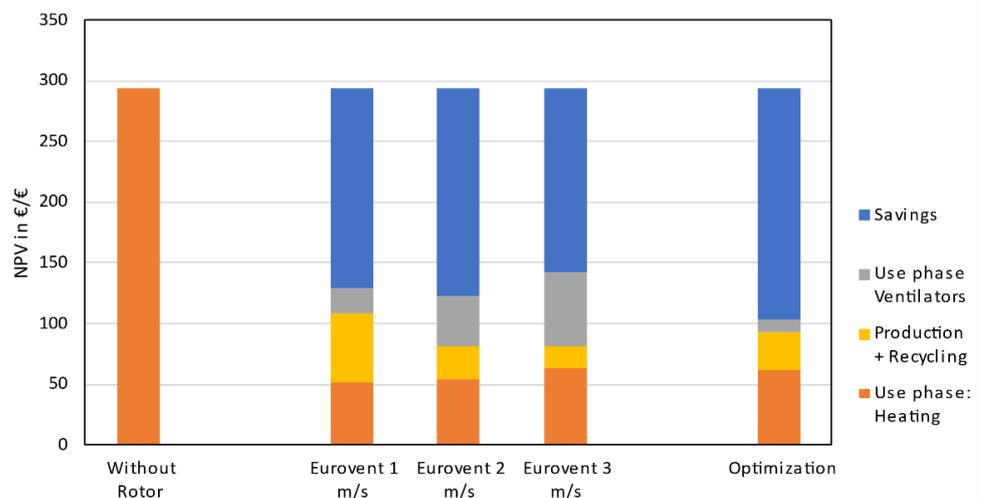
**Figure A2.** 25 €/t  $\text{CO}_2$  Eq. scenario with optimized RHX and Eurovent RHX under different operating ambient air empty tube velocities at  $100,000 \text{ m}^3/\text{h}$ .
