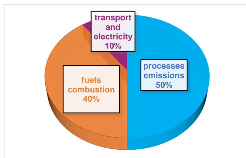
**Figure 1.** Operations in which CO<sub>2</sub> is generated in the OPC production process [49].
