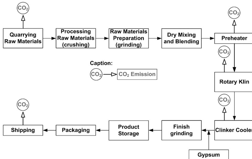
**Figure 2.** Detailed diagram showing the steps of OPC manufacturing and stages during which CO<sub>2</sub> is emitted [49].
