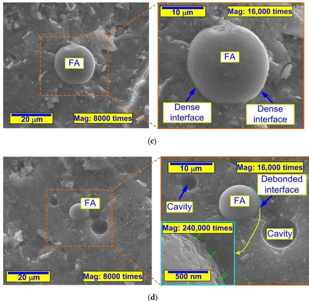
**Figure 3.** SEM micrographs of analyzed quaternary concretes including SCMs: (a) REF, (b) Q1, (c) Q2, (d) Q3; CH—calcium hydroxide, C-S-H—calcium silicate hydrate, E—ettringite, FA—fly ash.
