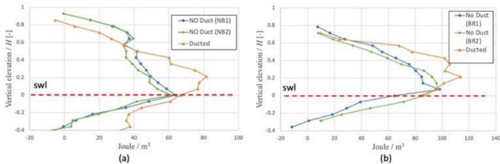
**Figure 15.** The energy per  $m^3$  of water comparison at (a) the near breaking wave zone of the no duct case at  $(x/L) = -0.175$ , (blue circle), no duct case at  $(x/L) = -0.25$  (green diamond), and the ducted case (orange triangle); and (b) the broken wave zone of the no duct case at  $(x/L) = 0.075$  (blue circle), no duct case at  $(x/L) = 0.125$  (green diamond) and ducted case (orange triangle). Here  $L$  denotes the shallow water wavelength.
