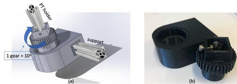
**Figure 7.** The (a) design in Solidworks® and (b) 3D printed angle switching mechanism for the wave angle ( $\beta$ ) exploration, where each gear rotation translates to a 10° rotation of the pressure transducer (PT) and physical model.
