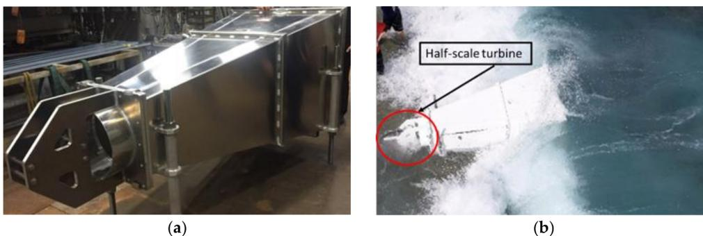
**Figure 3.** The early prototype of the duct design made from aluminum during fabrication (a); and during the field test (b). The model was painted white for protection against corrosion. The half-scale turbine was attached to the outlet of the duct during testing.
