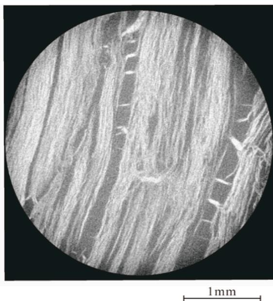
**Figure 4.** The 2D slice of coal 2-5 without fracture.
