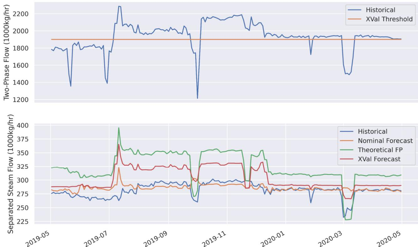
**Figure 10.** Results from a flash plant modeling cross-validation experiment where models were trained only with two-phase input mass flow less than 1900 tonne/h. The top plot shows the two-phase mass flow through FP16IP+ with the training data limitation. The bottom plot shows the historical separated steam flow compared to predictions by a baseline model trained on all data, the cross-validation (xval) model, and a theoretical model.
