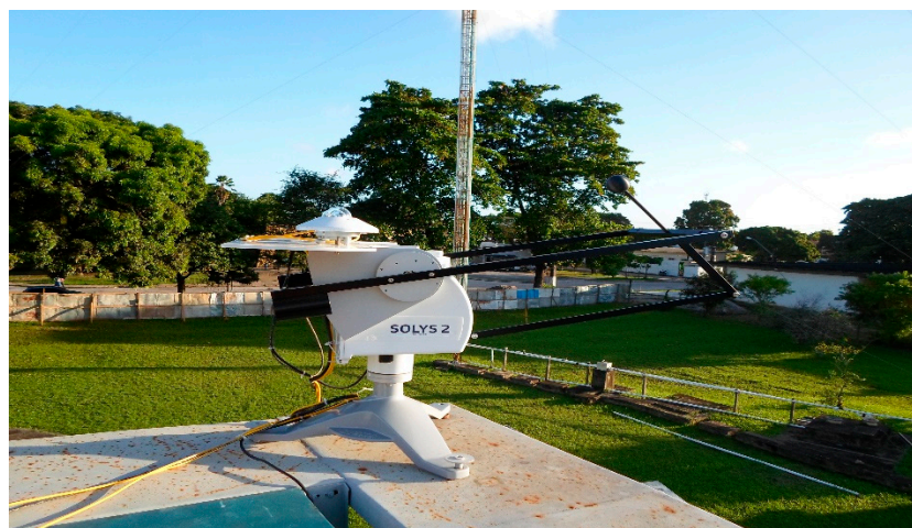
Figure 5. The solarimetric station for irradiance measurements.
