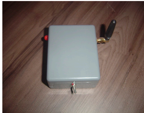
Figure 3. Radio frequency (RF) transceiver used in the computer to communicate with the solar tracker.
