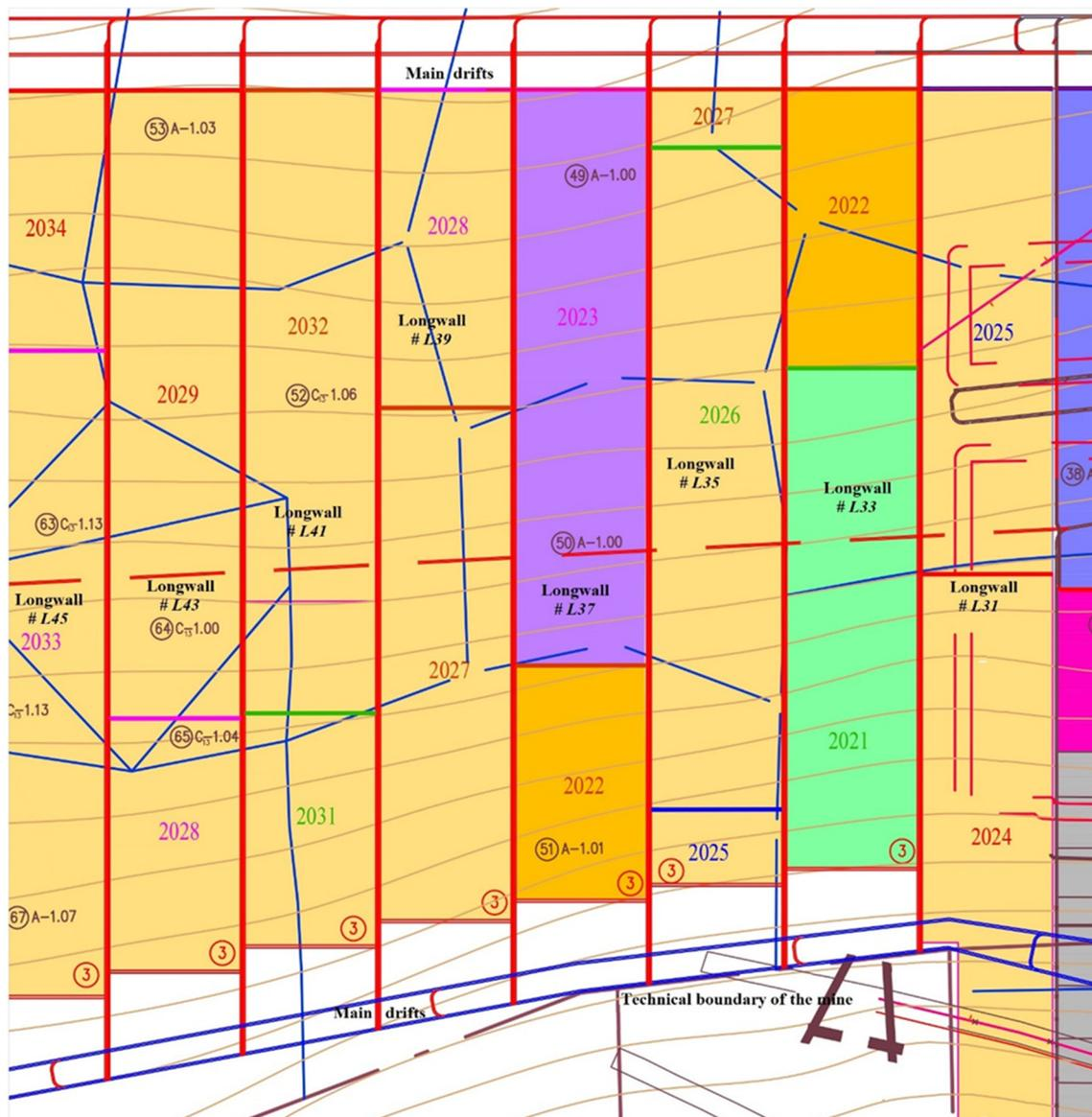
**Figure 2.** Plan of the mine field: 64 C $\pi$ 1.00—exploration well number with the indicated coal seam thickness; 2025—planned year of pillar exploration.
