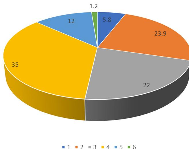
**Figure 1.** Schematic distribution of coal reserves according to their thickness in the context of “DTEK “Pavlohradvuhillia” PJSC mines: 1—<0.6 m; 2—0.61–0.7 m; 3—0.71–0.8 m; 4—0.81–1.0 m; 5—1.01–1.2 m; 6—>1.2 m [7,9].
