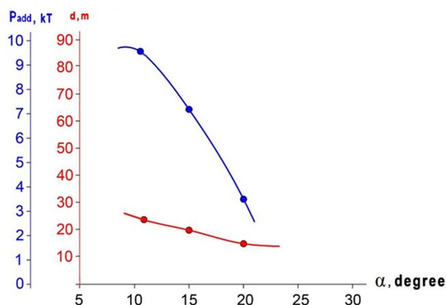
**Figure 4.** Dependence of the inclination angle of the break-down chamber on the distance to the permanent mine working and additional extraction from the extraction column area which is subject to robbing.
