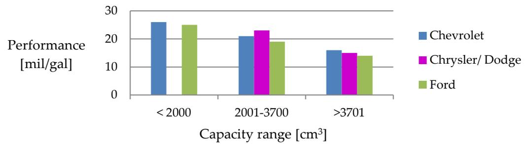
**Figure 13.** Performance in individual engine capacity ranges among American car brands. Source: Developed own.
