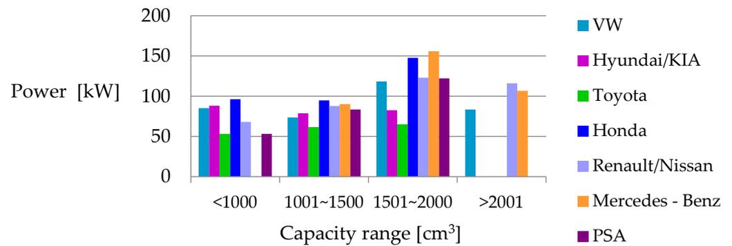
Figure 5. Engine power per liter of displacement in the different engine displacement compartments; European and Asian car brands. Source: Developed own.
