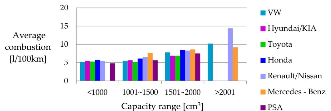
**Figure 4.** Average fuel consumption per engine capacity compartment; European and Asian car brands. Source: Developed own.
