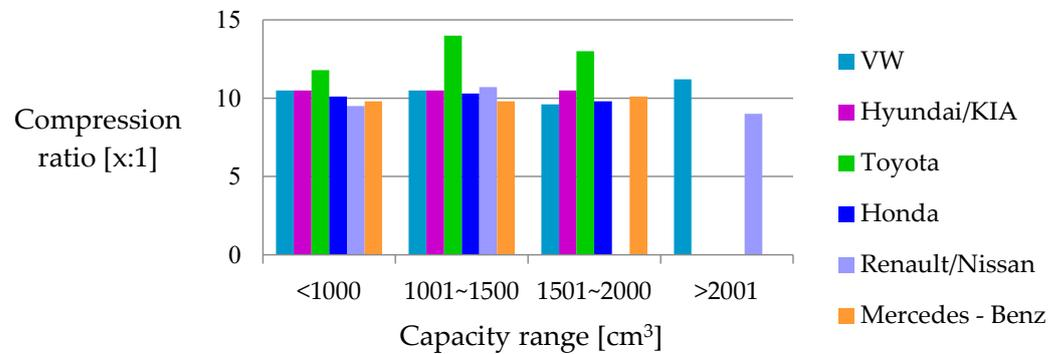
**Figure 3.** Compression ratio in the individual engine capacity compartments; European and Asian car brands. Source: Developed own.
