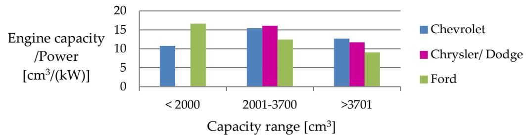
**Figure 15.** Ratio of engine capacity to power in individual engine capacity compartments among American car brands. Source: Developed own.
