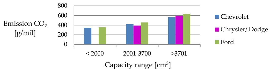
**Figure 14.** Carbon dioxide emissions in individual engine capacity ranges among American car brands. Source: Developed own.
