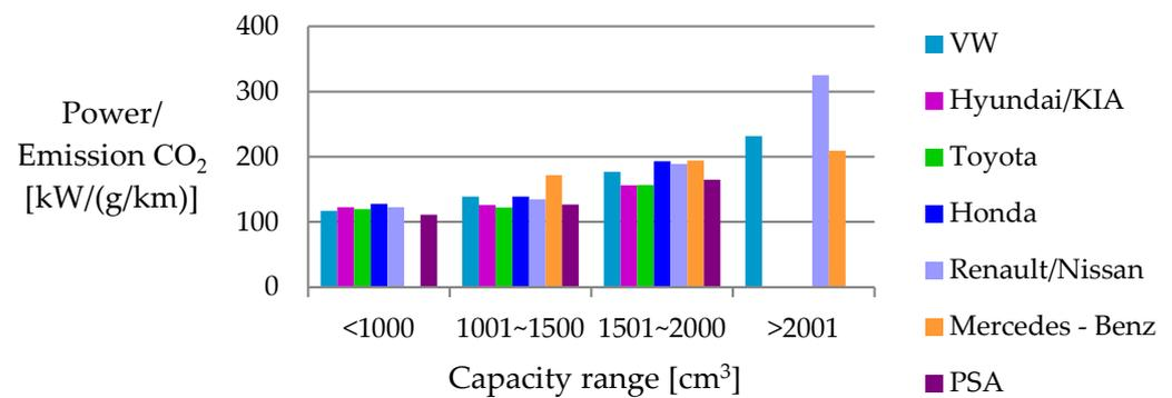
Figure 10. The ratio of maximum power to carbon dioxide emissions in the different engine capacity compartments; European and Asian car brands. Source: Developed own.
