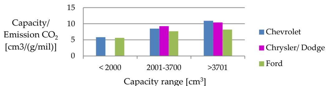
**Figure 17.** Ratio of capacity to carbon dioxide emissions in individual engine capacity ranges among American car brands. Source: Developed own.
