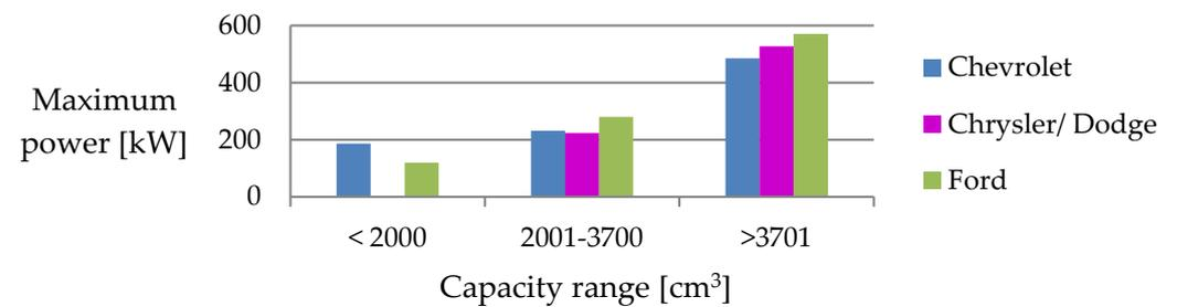
Figure 11. Maximum power in individual engine capacity ranges among American car brands. Source: Developed own.
