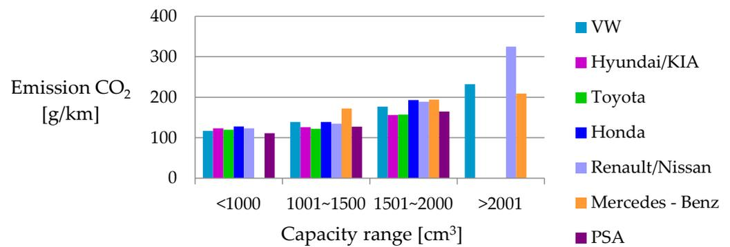
Figure 6. CO₂ emissions in individual engine displacement compartments; European and Asian car brands. Source: Developed own.
