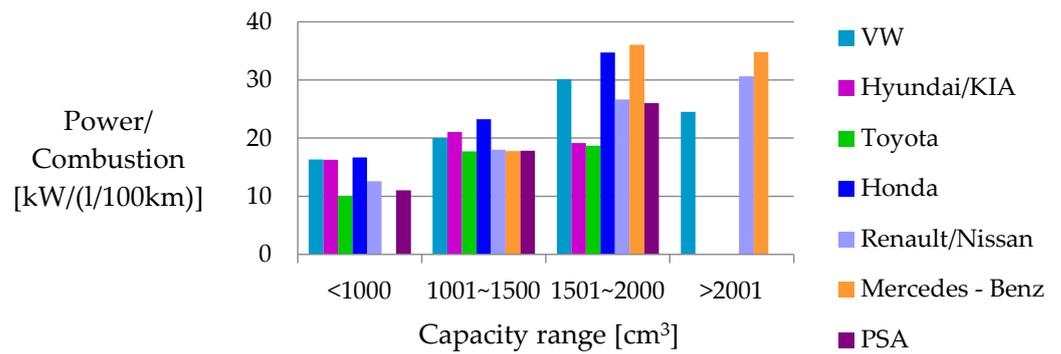
Figure 9. The ratio of maximum power to combustion in the individual engine capacity compartments; European and Asian car brands. Source: Developed own.
