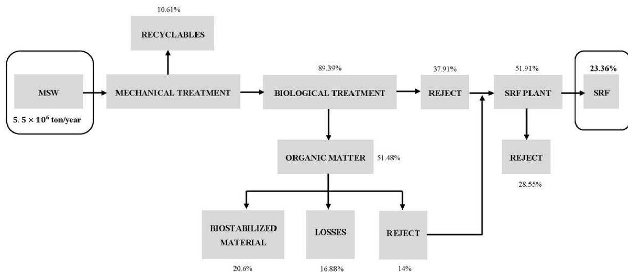
**Figure 4.** Flowchart of the process showing the mass balance (in % of the initial  $5.5 \times 10^6$  ton/year) [68].
